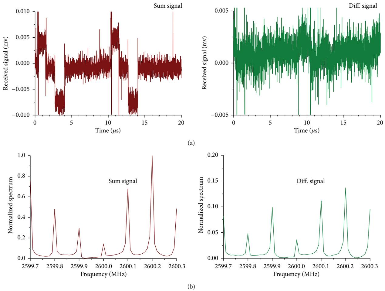
FIGURE 15: The procedure to obtain the difference-sum ratio  $K$ : (a) waveforms of sum and difference signals at  $\theta = 30^\circ$  and (b) spectra of sum and difference signals at  $\theta = 30^\circ$ .
