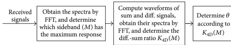
FIGURE 13: Signal processing steps in the 4D array for direction finding.
