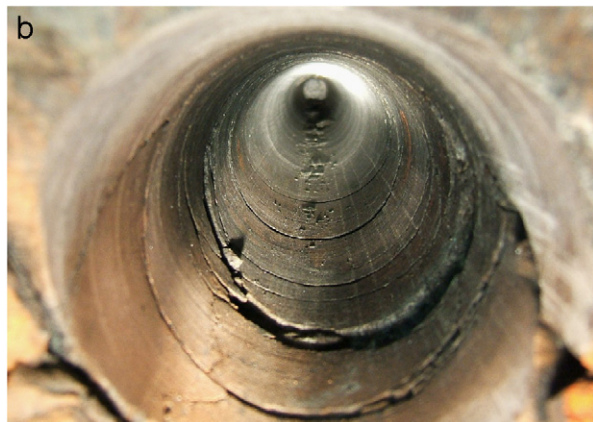
Fig. 2. (a) Surface parallel fractures observed from a cross-cut at Creighton Mine (depth 2500 m) in Canada and (b) surface parallel fractures revealed from a borehole (diameter = 10 cm) in highly stressed ground at Garson Mine in Canada (depth 1500 m; the maximum principal stress is roughly horizontal, and the intermediate principal stress vertical).
