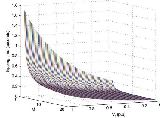
Fig. 1. Proposed relay time–current–voltage characteristic with  $K = 2$  and  $TDS = 0.1$ .
