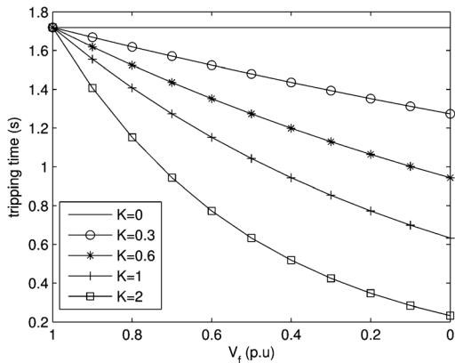
Fig. 2. Effect of the setting  $K$  on the proposed relay tripping time with  $M = 1.5$  and  $TDS = 0.1$ .
