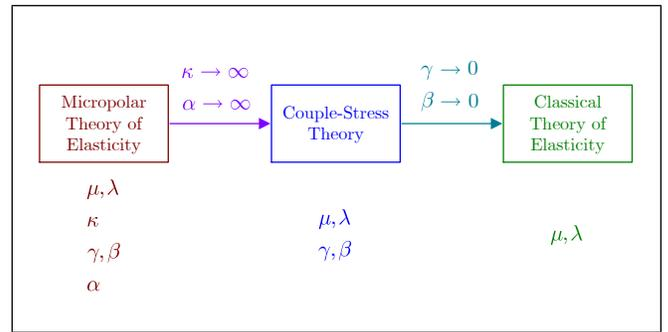
**FIGURE 3.** SEQUENTIAL STRUCTURE FOR SIMPLIFICATION OF THE MICROPOLAR ELASTICITY THEORY TO THE COUPLE-STRESS AND CLASSICAL ELASTICITY THEORIES.
