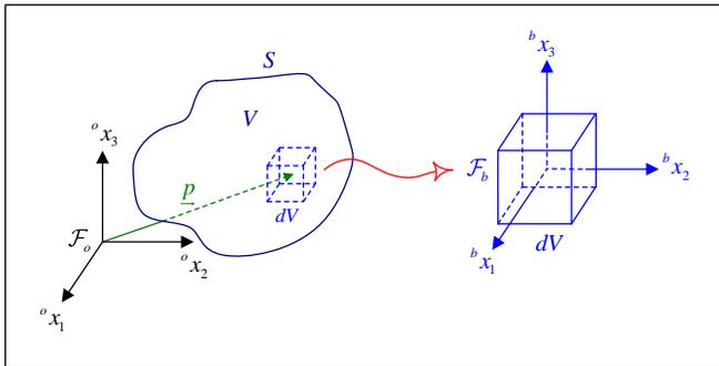
**FIGURE 1.** A GENERAL ELASTIC BODY AND ITS REPRESENTATIVE ELEMENT.
