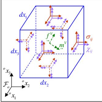
**FIGURE 2.** FREE BODY DIAGRAM OF A REPRESENTATIVE ELEMENT IN A MICROPOLAR ELASTIC BODY.
