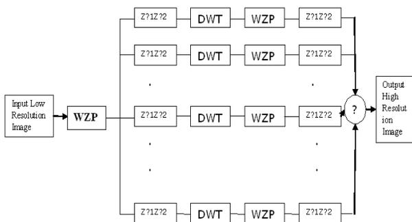
**Fig3. Block Diagram of the WZP-and-CS-based image Resolution Enhancement [4].**
