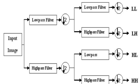
Fig 1. Block diagram of DWT Filter Banks of level 1 [8]
