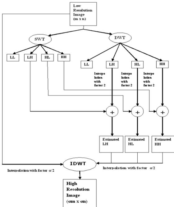
Fig 6. Block diagram of image resolution enhancement method using SWT and DWT [7].
