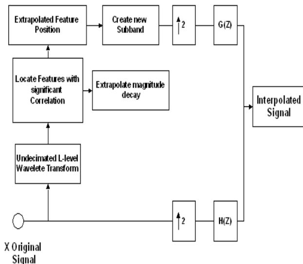
Fig 2. Block diagram of interpolation system for 1-D row and column signals[2].
