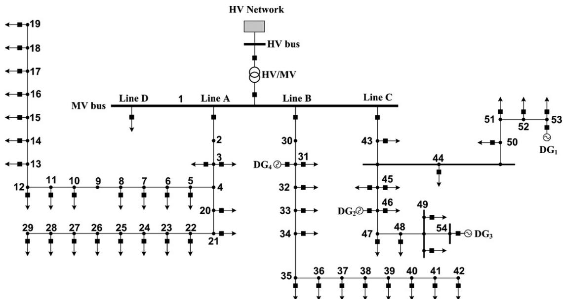
Fig. 3. Italian radial network for test case.
