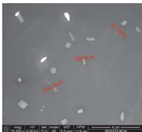
Figure 4 SEM image of polymeric film with CaO.
