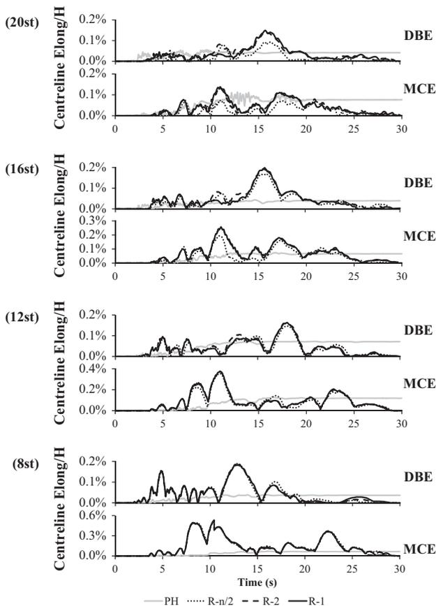
Fig. 11. The average of maximum centerline elongation of rocking walls under the DBE and MCE record.
