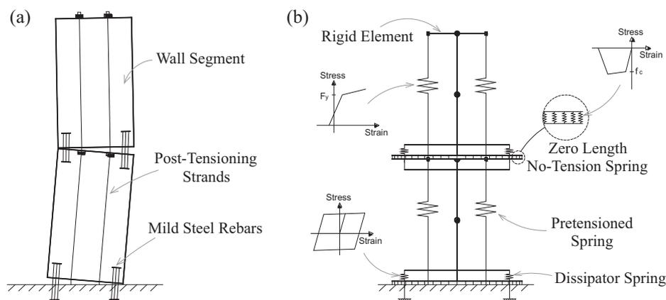
Fig. 1. Multiple rocking system (a) physical model, (b) analytical model and component behavior.
