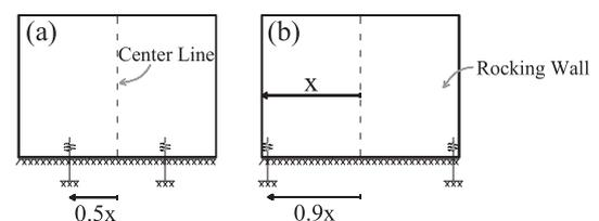
**Fig. 6.** Location of the energy dissipation and post-tensioning tools (a) 0.5x mode, (b) 0.9x mode.
