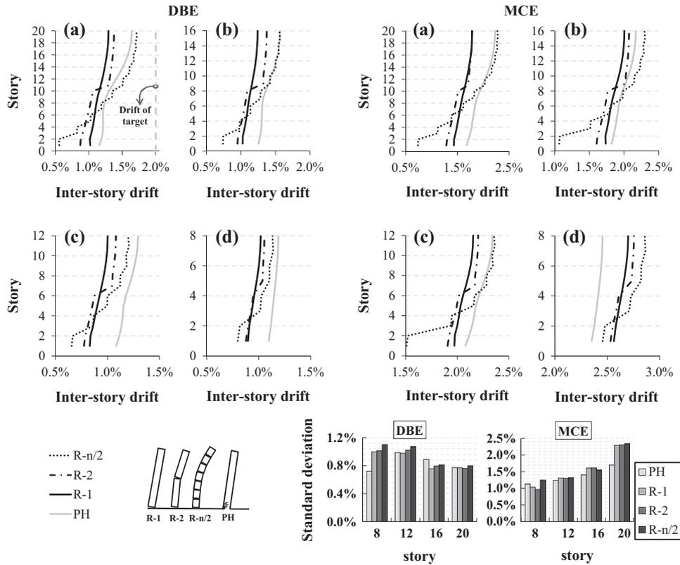
Fig. 9. The results of average of maximum inter-story drift under the DBE and MCE records.
