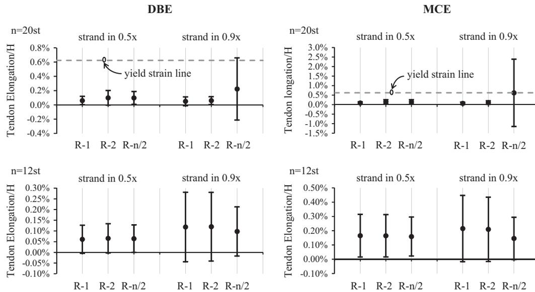
Fig. 8. The results of the average of maximum strand elongation and dispersions for 0.5x and 0.9x models under the DBE and MCE records.
