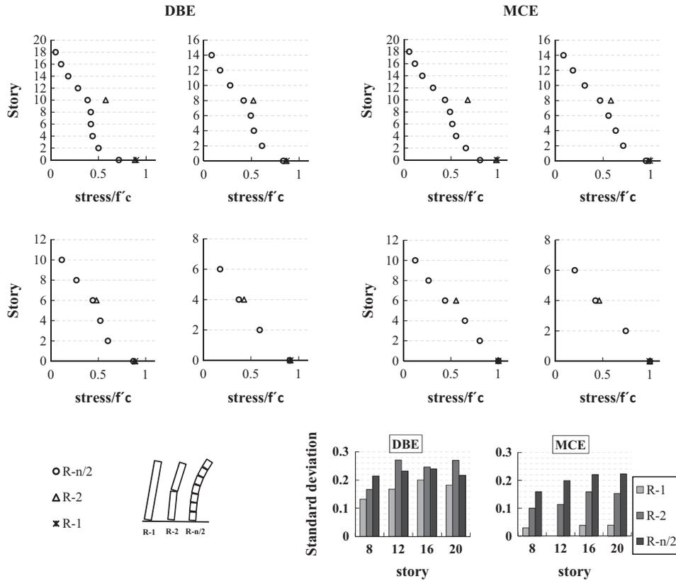
Fig. 14. The mean of maximum stresses of concrete at edges of rocking sections under DBE and MCE records.
