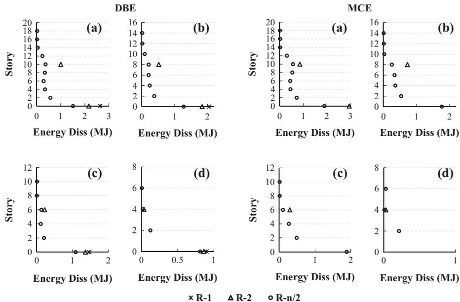
Fig. 15. The mean of cumulative energy dissipation at rocking sections under the DBE and MCE records (units are Mega Joule).
