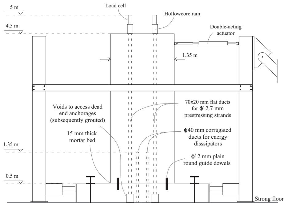
Fig. 2. The test setup and specimen adopted from [21].
