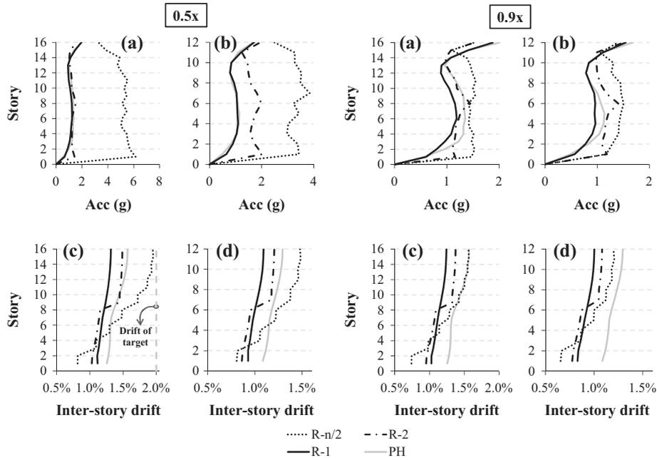
Fig. 7. The results of the average of maximum horizontal acceleration and inter-story drift for 0.5x and 0.9x models of energy dissipation tools under the DBE record.
