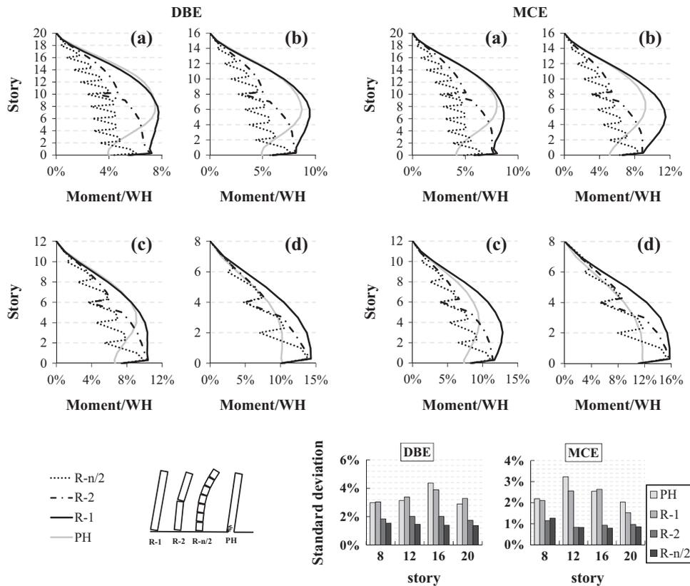
Fig. 13. The mean of maximum bending moment under the DBE and MCE record.
