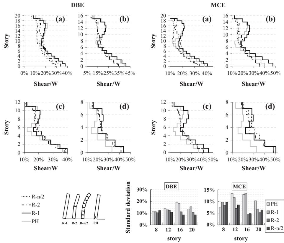
Fig. 12. The average of maximum shear forces under DBE and MCE record.
