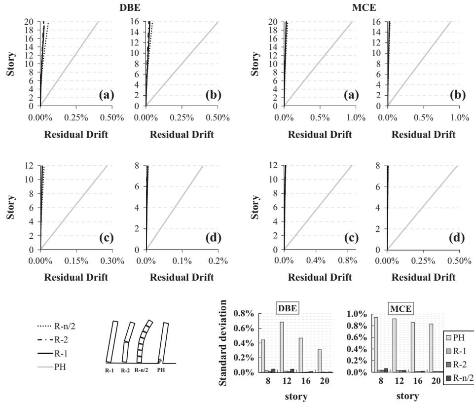
Fig. 10. The results of the average maximum residual drift under DBE and MCE records.
