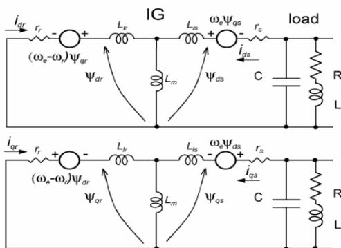
Fig.1 d-q axes equivalent circuit of SEIG
