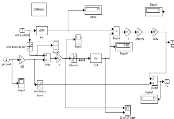
Fig. 5 Custom wind turbine model (Air Density: 1.1 kpa)
