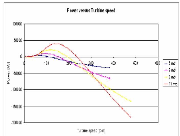
Fig. 6 Output Mechanical Power of Turbine versus the Turbine Speed
