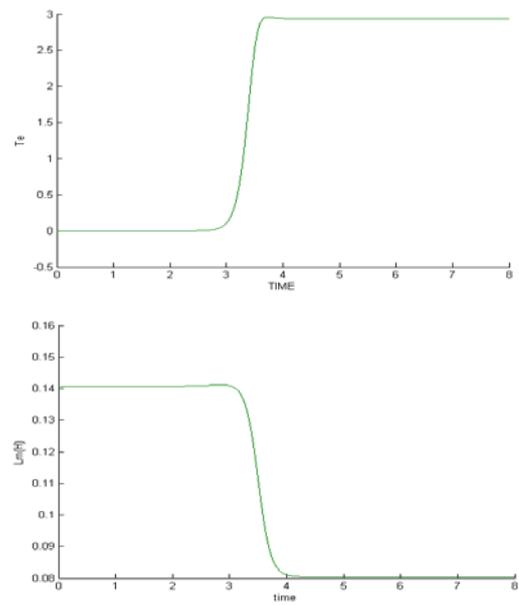
Fig. 8. SEIG at RLC-load with constant excitation (graphs: 1. Stator line voltages 2.Stator currents 3. Load currents 4.Capacitor currents. 5. Electromagnetic torque 6.Magnetizing inductance)
