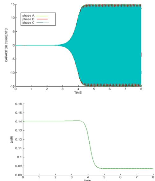
Fig.9. SEIG at RLC-load with constant excitation (graphs: 1. Stator line voltages 2.Stator currents 3. Load currents 4.Capacitor currents. 5. Electromagnetic torque 6.Magnetizing inductance)
