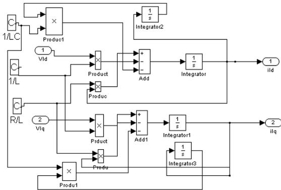
Fig.2 SIMULINK model of RLC load
