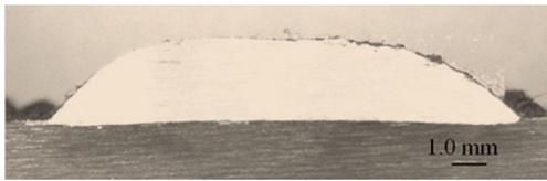
**Fig. 16** Cross section of the clad deposited under the optimal operative conditions
