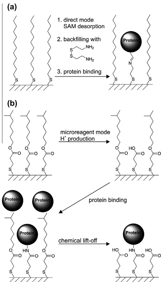
**Fig. 3.** Scanning electrochemical microscopy (SECM) allows for localized biomolecule attachment in the direct and microreagent modes of operation. Patterning schemes according to: (a) [62]; and, (b) [54].
