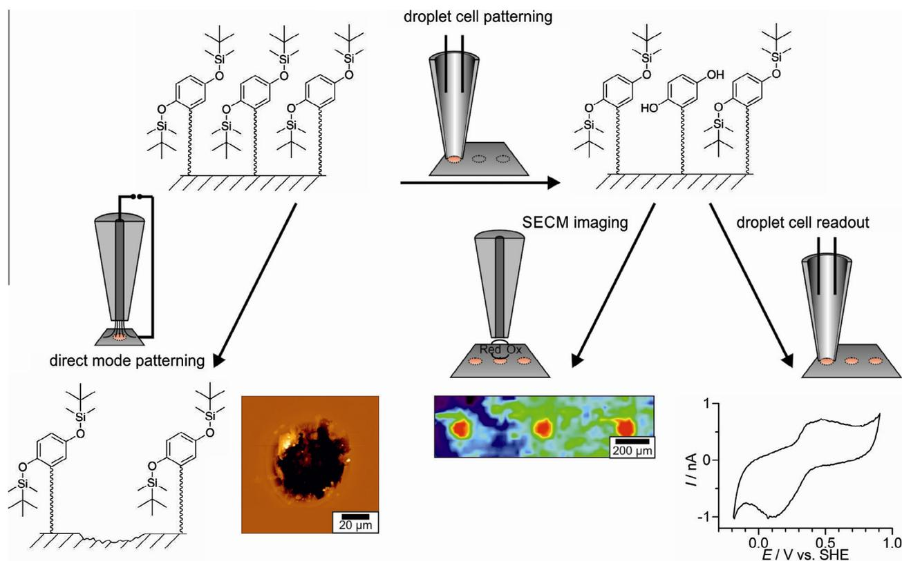
**Fig. 4.** The scanning droplet cell is used for truly chemoselective patterning. Direct mode SECM patterning results in substrate corrosion (AFM image, left branch). The droplet cell yields successful localized electrochemical cleavage of the TBDMOS protecting group as confirmed by SECM imaging and locally recorded cyclic voltammograms showing the typical redox signals for the surface-confined quinone groups (right branch) [68].
