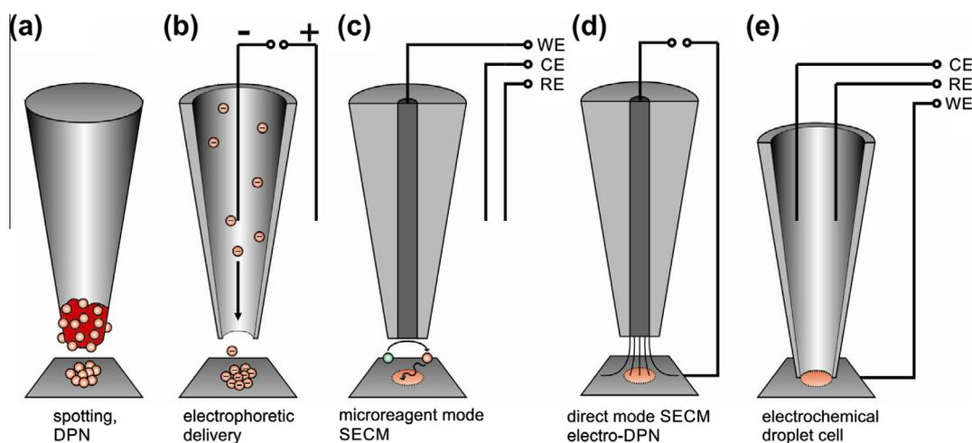
**Fig. 2.** Scanning probe techniques in various configurations are employed to induce local surface modifications. Patterning schemes as for: (a) spotting/DPN; (b) electrophoretic delivery; (c) microreagent mode SECM; (d) direct mode SECM/electro-DPN; and, (e) the electrochemical droplet cell.
