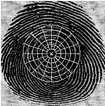
Figure 3: Reference point ( \times ), the region of interest and 80 sectors superimposed on a fingerprint.
