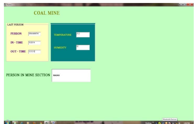
Fig.8: Values of sensor and in time and out time of person RFID card 1
