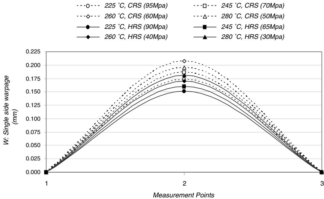
Fig. 9. Comparison of the minimum single side warpages for ABS vs. temperature and pressure when using both HRS and CRS.
