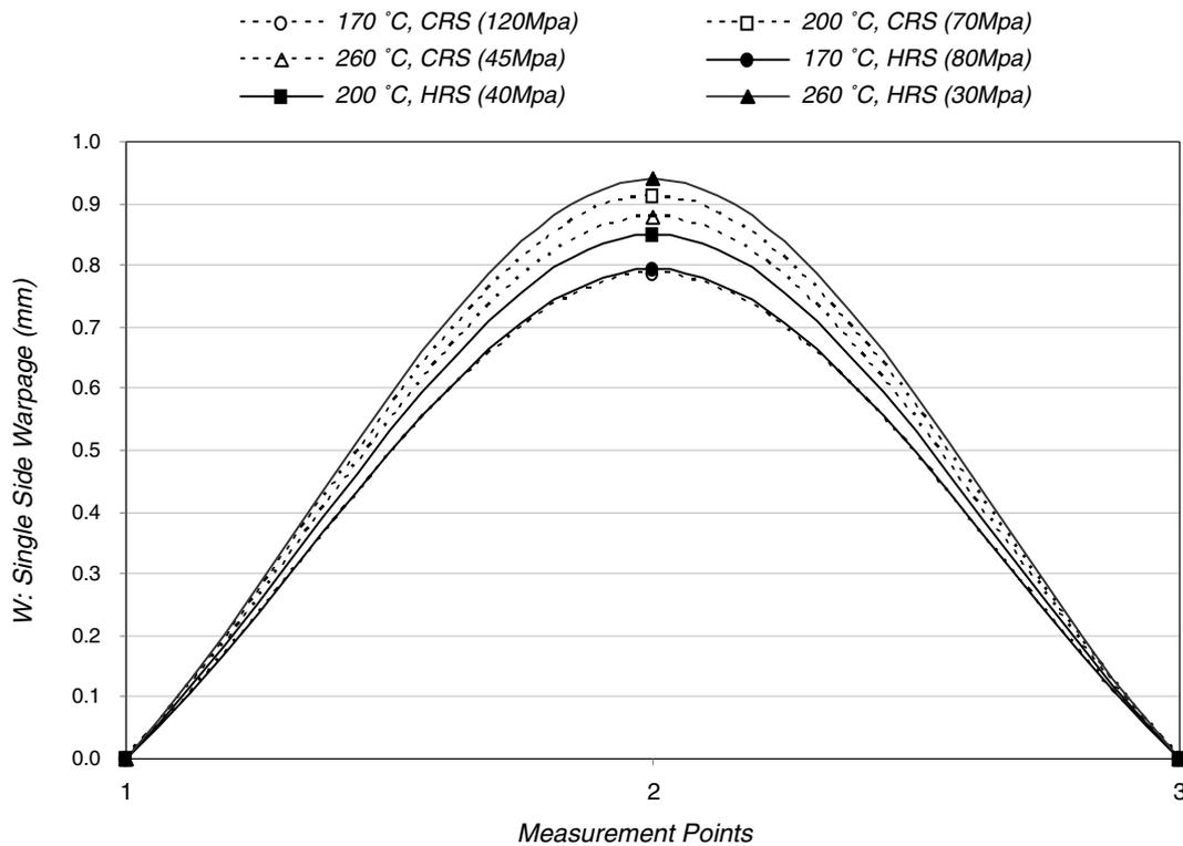
Fig. 10. Comparison of the minimum single side warpages for PP material vs. temperature and pressure when using both HRS and CRS.
