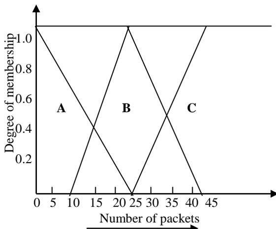
Figure 2. Fuzzy space used in Intrusion Detection
