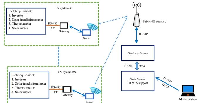
Fig. 3. Communication topology of REMS.
