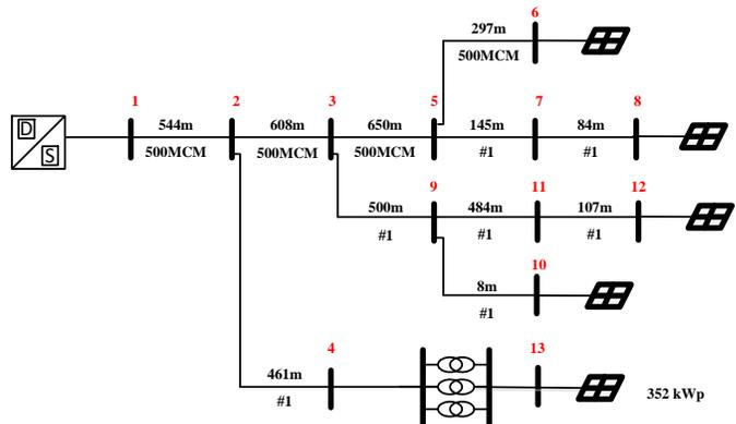
Fig. 6. One-line diagram of test feeder RA11.
