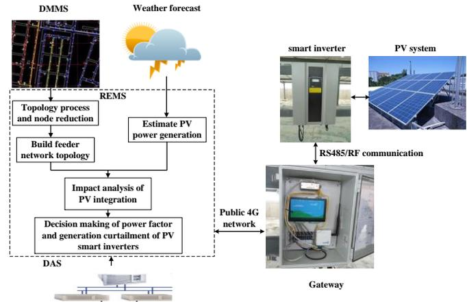
Fig. 2. Function block diagram of the REMS.
