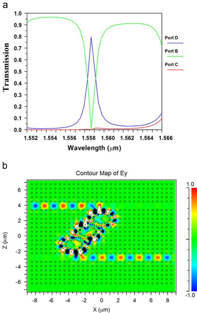
**Fig. 9.** (a) The output spectrum of the CDF with triple ring and (b) Distribution of optical power at  $\lambda = 1559 \text{ nm}$ .
