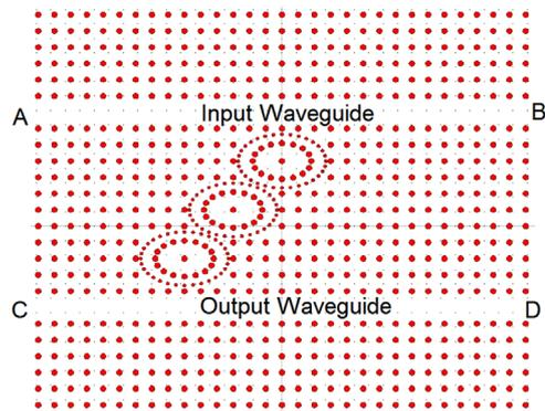
Fig. 7. The schematic diagram of the proposed CDF with triple resonant ring.
