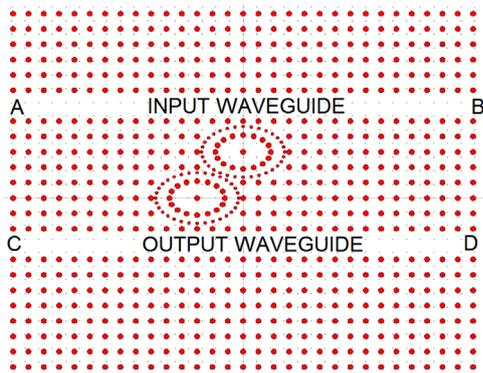
Fig. 6. The schematic diagram of the proposed CDF with dual resonant ring.
