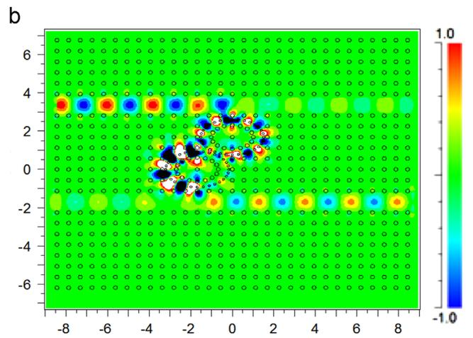
Fig. 8. (a) The output spectrum of the CDF with dual ring and (b) Distribution of optical power at  $\lambda=1558$  nm.
