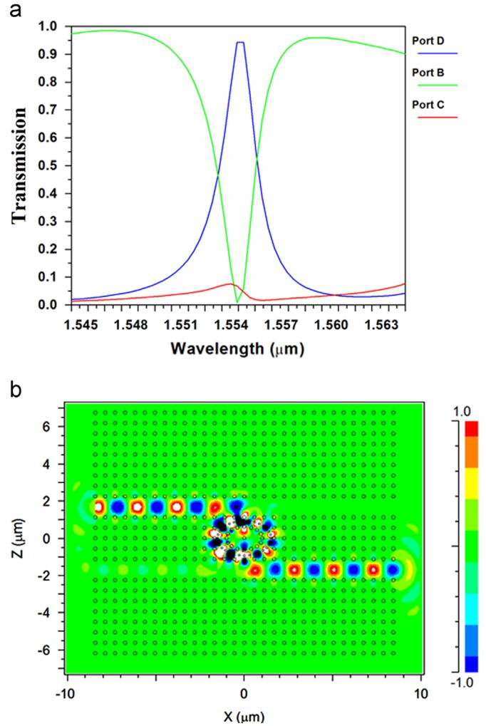
Fig. 3. (a) The output spectrum of the proposed CDF and (b) Distribution of optical power at  $\lambda = 1555$  nm. (For interpretation of the references to color in this figure, the reader is referred to the web version of this article.)
