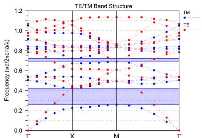
Fig. 1. The band structure of the basic PhC structure. (For interpretation of the references to color in this figure, the reader is referred to the web version of this article.)
