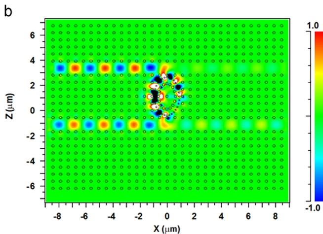
Fig. 5. (a) The output spectrum of the CDF with vertical ring and (b) Distribution of optical power at  $\lambda=1550$  nm.
