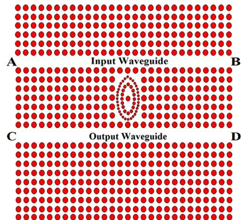
Fig. 4. The schematic diagram of the proposed CDF with vertical resonant ring.
