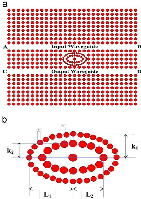
Fig. 2. The schematic diagram of (a) the proposed CDF (b) and its resonant ring.
