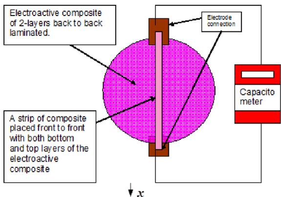
Fig. 4. Test piece structure of pressure sensor: Model 2/3
