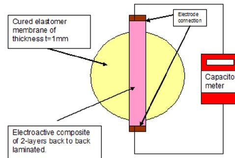
Fig. 6. Test piece structure of pressure sensor: Model 3/3
