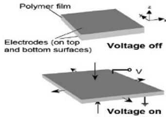
Fig. 1. Applying voltage to the electrodes makes the electronic EAP's change its shape
