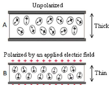
Fig. 2. With an electric field aligning the dipoles in the dielectric, the electrostrictive forces pull the material together
