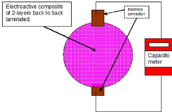
Fig. 3. Test piece structure of pressure sensor: Model 1/3
