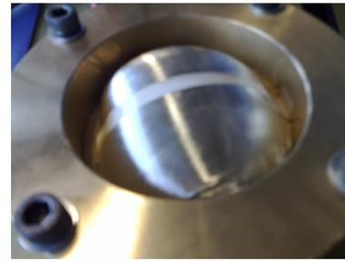
Fig. 5. Deformation of the test piece (Model 2/3) structure under pressure effect
