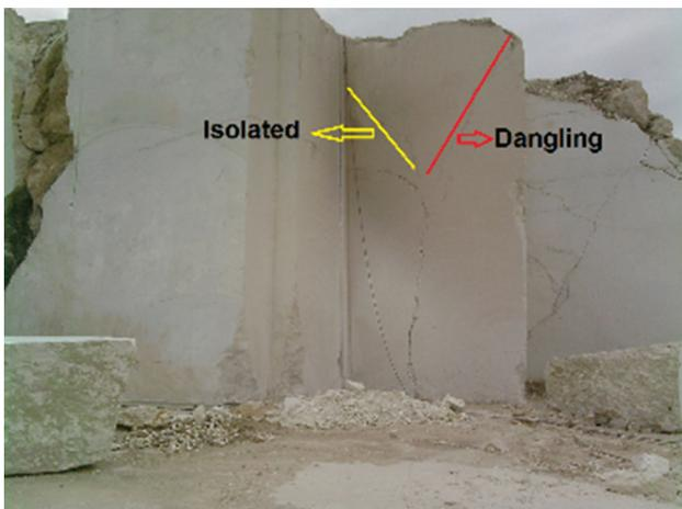
Fig. 2 Dangling and isolated discontinuities in a step face in Joshaqan quarry
