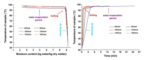
Fig. 4. Temperature of tomato samples during ohmic heating.
