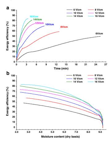
Fig. 10. Variation of exergy efficiency as a function of (a) time, (b) moisture content.
