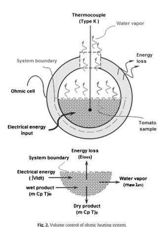
The energy efficiency of the ohmic heating system was determined in Eq. (8);
