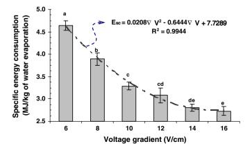
**Fig. 7.** Amount of specific energy required for ohmic heating of tomato samples. <sup>a–e</sup> Different superscripts in the same column indicate significant differences (P < 0.05).
