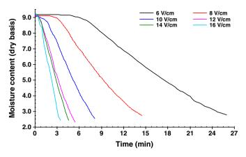
Fig. 3. Variations of moisture content as a function of time for different voltage gradient.
