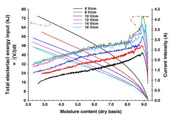
Fig. 8. Variation of electrical energy input and current intensity at different voltage gradients.
