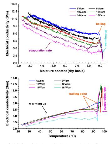
Fig. 9. Electrical conductivity changes of the tomato samples during ohmic heating.
