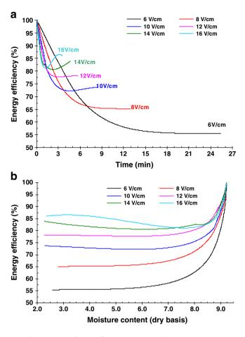
Fig. 5. Variation of energy efficiency with (a) time, (b) moisture content.
