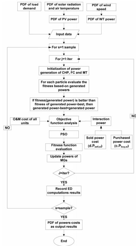
Fig. 3. Flowchart of implementation of PSO on probabilistic ED.
