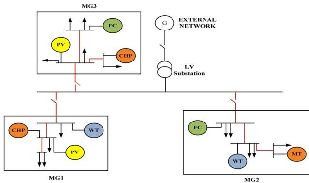
Fig. 1. Structure of network with three MGs (SSEZ).
