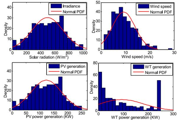
Fig. 5. Probabilistic modeling of PV and WT primary input and generated power in MG1.
