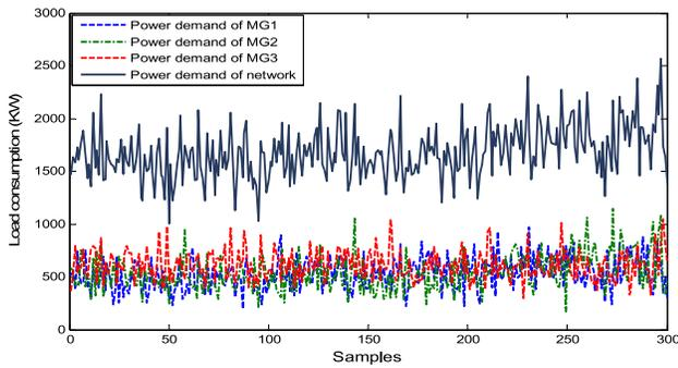
Fig. 4. Load demand of MGs 1, 2, and 3 and network.
