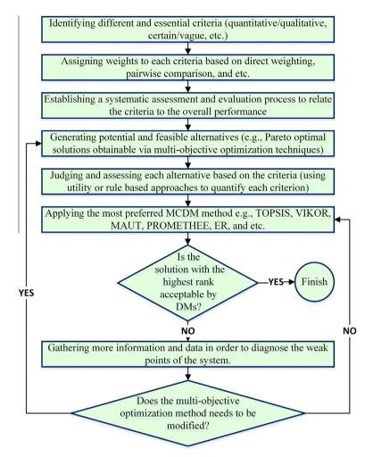
Fig. 2. Framework outlining the amalgamation of MCDM with multi-objective optimization methods.
