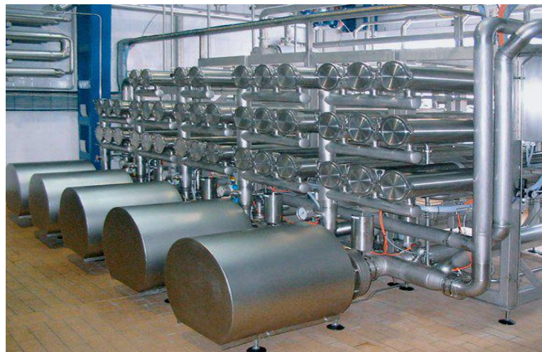
Picture 1. The overview of a UF unit for whey
