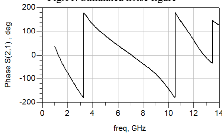
Fig. 12: Simulated phase shift vs frequency
