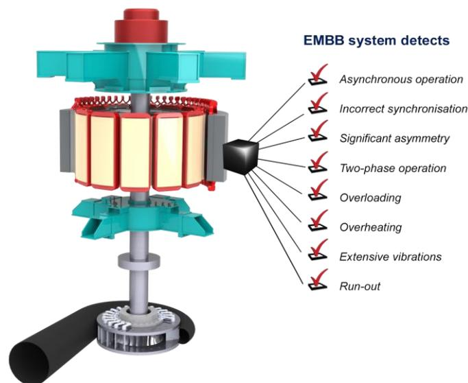
Fig. 1. Harmful working conditions EMBB system detects.
