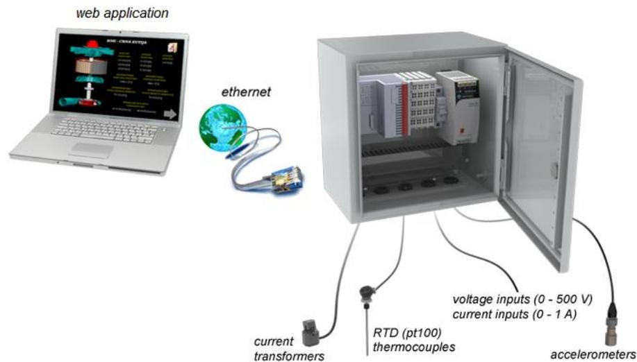
Fig. 2. EMBB system concept and design.
