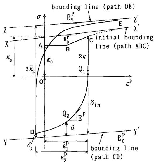
Figure 1 Uniaxial stress  $\sigma$ –plastic strain  $\epsilon^p$  curve
