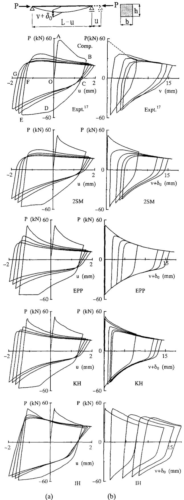
Figure 6 Comparison between predicted and experimental results: (a) axial load  $P$ –axial displacement  $u$ ; (b) axial load  $P$ –midspan deflection  $v$ . ( $KL/r = 40.46$ ,  $L = 174$  mm,  $b = 15.45$  mm,  $h = 14.90$  mm,  $\delta_0 = 0.1\%L$ ,  $\sigma_y = 229.0$  MPa,  $E = 206.7$  GPa,  $\epsilon_{st}^p = 0.8\%$ )
