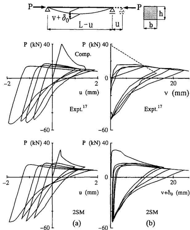
Figure 9 Comparison between predicted and experimental results: (a) axial load  $P$ -axial displacement  $u$ ; (b) axial load  $P$ -midspan deflection  $v$ . ( $KL/r=120.66$ ,  $L=521$  mm,  $b=15.42$  mm,  $h=14.96$  mm,  $\delta_0=0.1\%L$ ,  $\sigma_y=229.0$  MPa,  $E=206.7$  GPa,  $\epsilon_{sr}^p=0.8\%$ )
