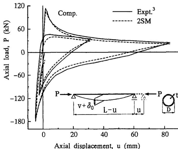
Figure 10 Comparison between predicted and experimental results; axial load  $P$ -axial displacement  $u$ . ( $KL/r=115$ ,  $L=2300$  mm,  $D=60.33$  mm,  $t=3.91$  mm,  $\delta_0=0.1\%L$ ,  $\sigma_y=379.0$  MPa,  $E=197.0$  GPa)
