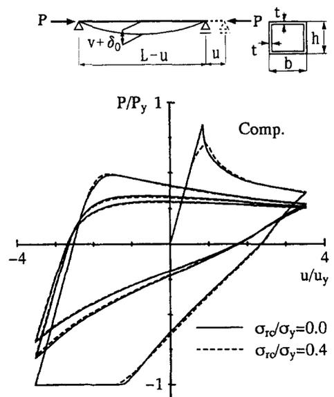
Figure 13 Effect of residual stress; normalized axial load  $P/P_y$ -axial displacement  $u/u_y$  for a pin-ended tubular column. ( $KL/r = 70$ ,  $L = 3150$  mm,  $b = 150.0$  mm,  $h = 110.0$  mm,  $t = 4.5$  mm,  $\delta_0 = 0.1\%L$ ,  $\sigma_y = 265.9$  MPa,  $E = 197$  GPa,  $\epsilon_{st}^p = 10\epsilon_y$ ,  $\sigma_{rt} = \sigma_y$  and  $\sigma_{rc} = 0.4\sigma_y$ )
