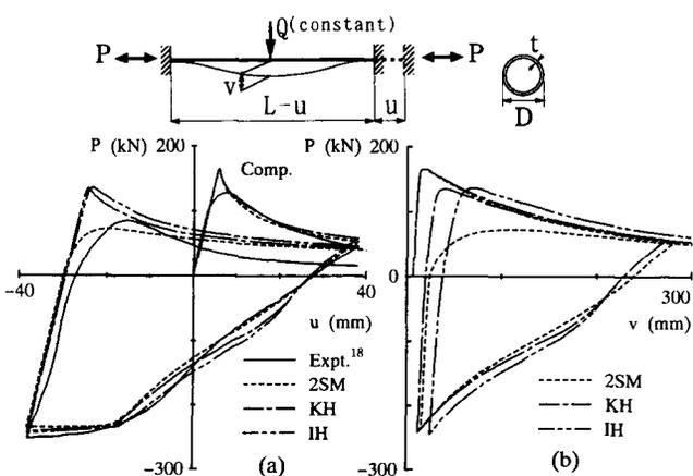
Figure 12 Comparison between predicted and experimental results: (a) axial load  $P$ -axial displacement  $u$ ; (b) axial load  $P$ -midspan deflection  $v$ . ( $KL/r = 72$ ,  $Q = 0.2Q_y$ ) (key as in Figure 11)
