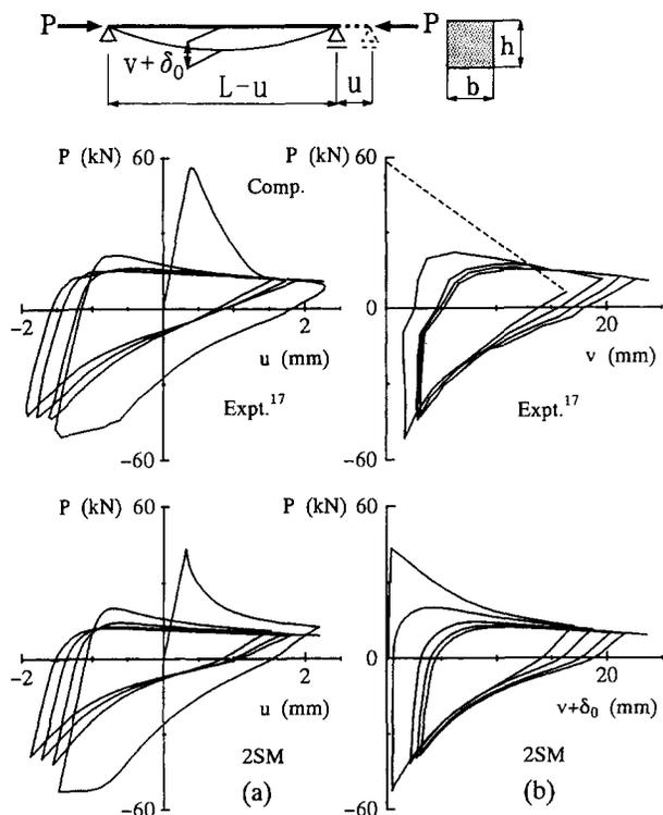
Figure 8 Comparison between predicted and experimental results: (a) axial load  $P$ -axial displacement  $u$ ; (b) axial load  $P$ -midspan deflection  $v$ . ( $KL/r=80.23$ ,  $L=349$  mm,  $b=15.21$  mm,  $h=15.07$  mm,  $\delta_0=0.1\%L$ ,  $\sigma_y=229.0$  MPa,  $E=206.7$  GPa,  $\epsilon_{sr}^p=0.8\%$ )
