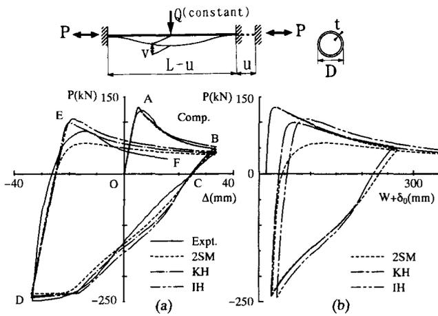
Figure 11 Comparison between predicted and experimental results: (a) axial load  $P$ -axial displacement  $u$ ; (b) axial load  $P$ -midspan deflection  $v$ . ( $KL/r = 72$ ,  $L = 5720$  mm,  $D = 114.0$  mm,  $t = 2.3$  mm,  $\sigma_y = 289$  MPa,  $Q = 0.4Q_y$ ,  $Q_y = 9.12$  kN,  $E = 200.0$  GPa)
