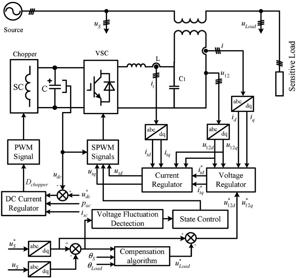
Fig. 2. Block diagram of the DVR controller.
