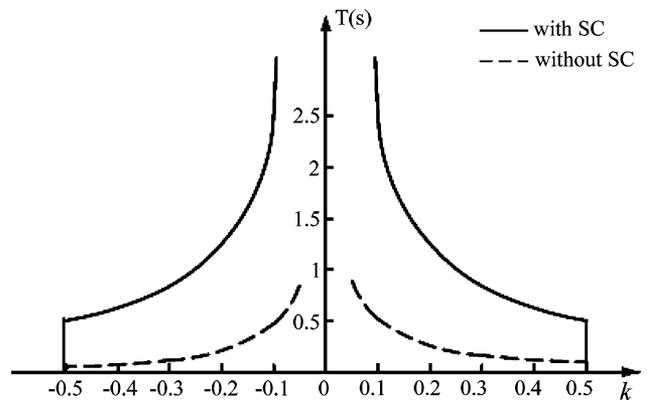
Fig. 3. The comparison of the compensation scope for a DVR with and without the superconducting magnet.
