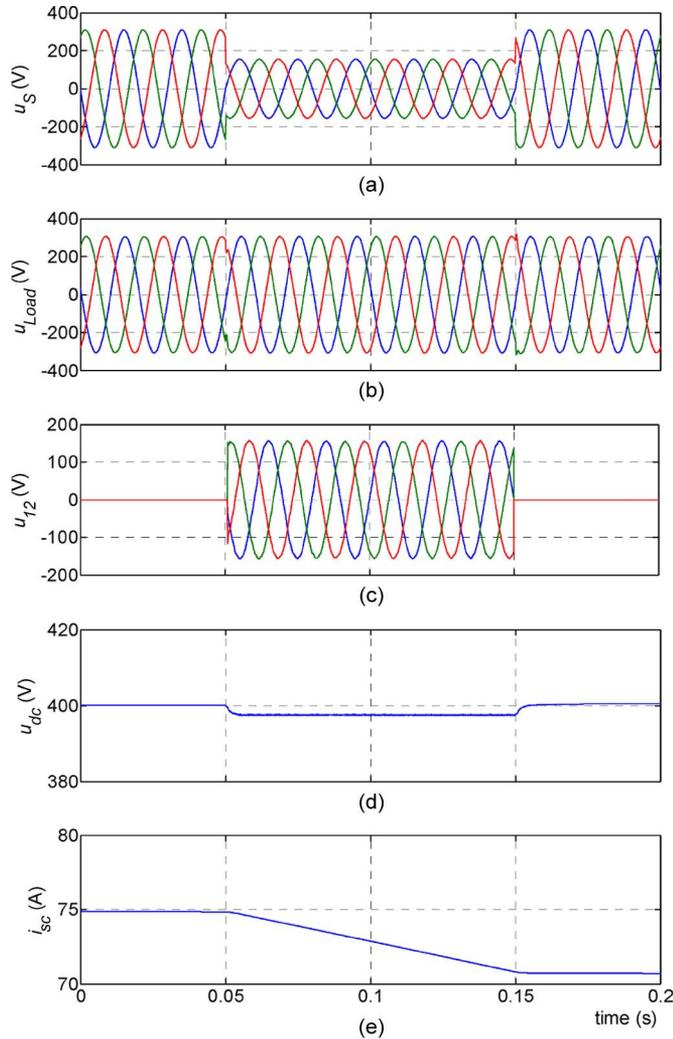
Fig. 4. Dynamic compensation for voltage sag.
