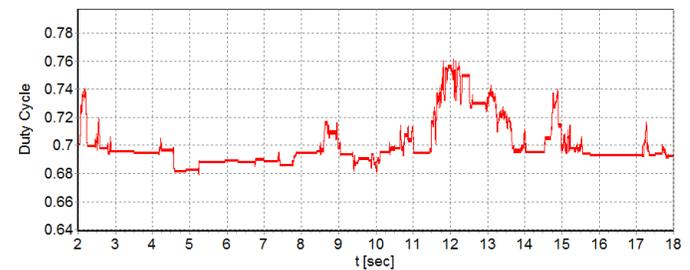
Figure 19 – Duty cycle of the MPPT module
