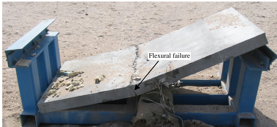
Fig. 16. Flexural failure of the RUHPFC specimen.
