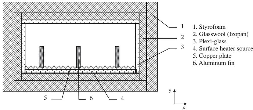
Fig. 2. Cross-section view of the channel.
