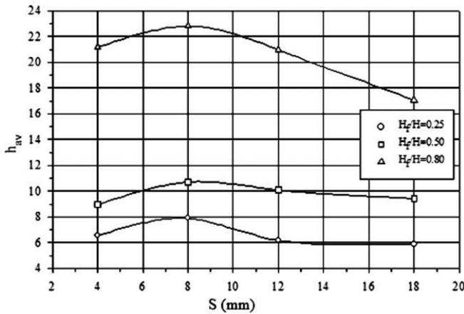
**Fig. 3.** Variation of average convection heat transfer coefficient with fin spacing at different fin heights (average modified Rayleigh number,  $Ra^* = 4 \times 10^7$ ).
