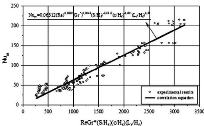
Fig. 19. Comparison of the correlation obtained from the present study with experimental results.
