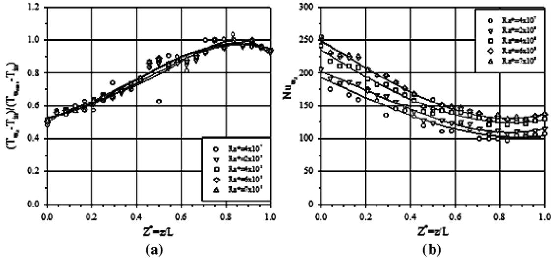
Fig. 18. (a) Variation of the temperature distribution and (b) variation of Nusselt Number with the main flow direction ( $z$ ) ( $S/H = 0.08$  and  $H_f/H = 0.80$ ).
