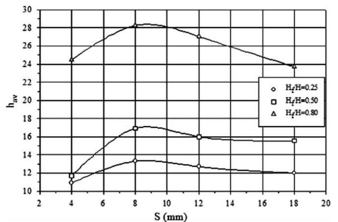
**Fig. 7.** Variation of average convection heat transfer coefficient with fin spacing at different fin heights (average modified Rayleigh number,  $Ra^* = 7 \times 10^8$ ).
