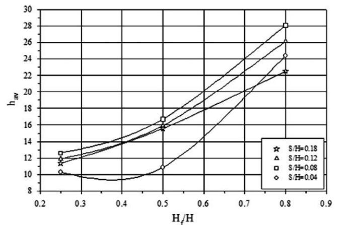
Fig. 11. Variation of average convection heat transfer coefficient with fin height at different fin spacings (average modified Rayleigh number,  $Ra^* = 6 \times 10^8$ ).
