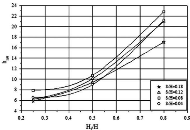
Fig. 8. Variation of average convection heat transfer coefficient with fin height at different fin spacings (average modified Rayleigh number,  $Ra^* = 4 \times 10^7$ ).
