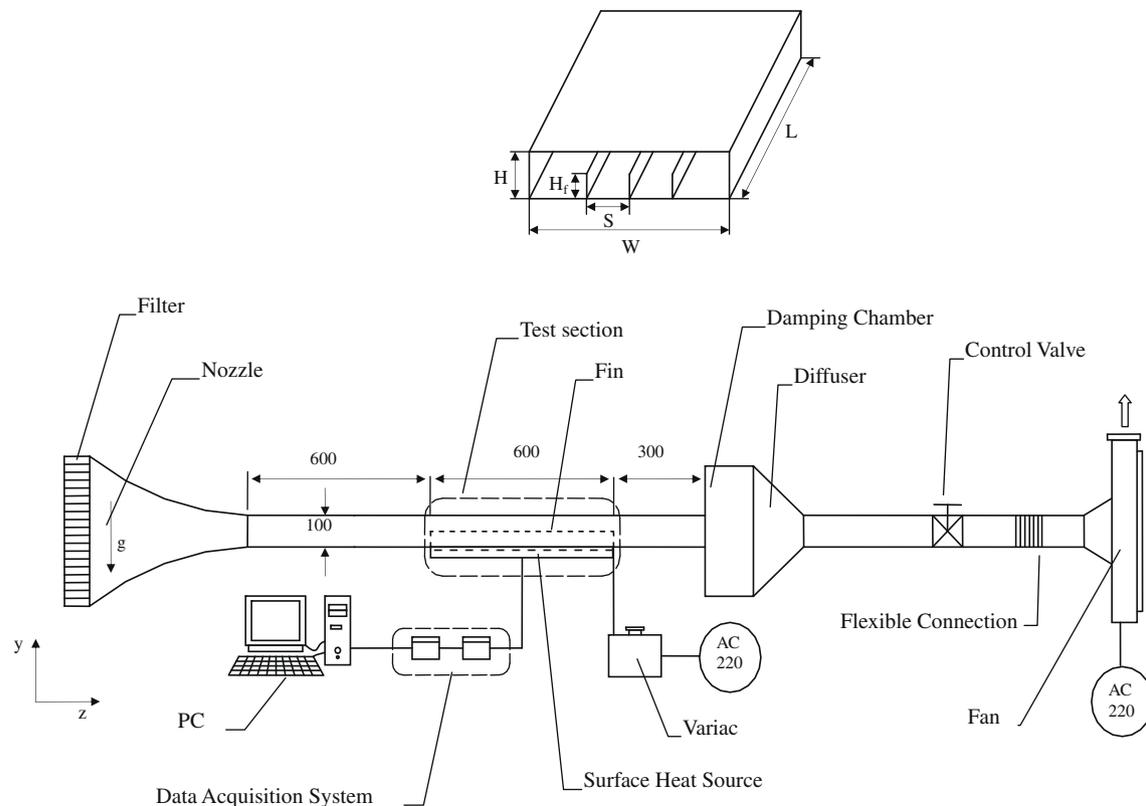
Fig. 1. Schematic diagram of the experimental set-up, (measures are in mm).
