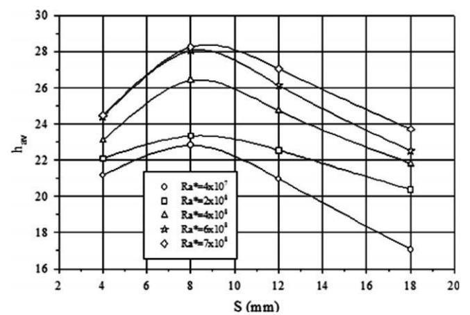
Fig. 15. Variation of average convection heat transfer coefficient with fin spacing (fin height,  $H_f/H = 0.80$ ).
