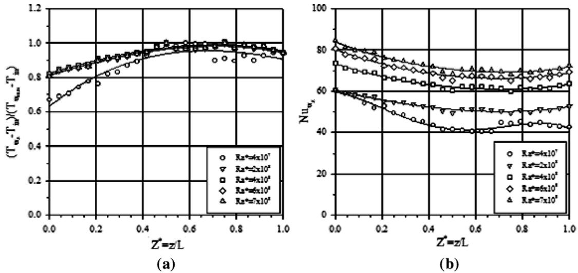
Fig. 16. (a) Variation of the temperature distribution and (b) variation of Nusselt Number with the main flow direction ( $z$ ) ( $S/H = 0.08$  and  $H_f/H = 0.25$ ).
