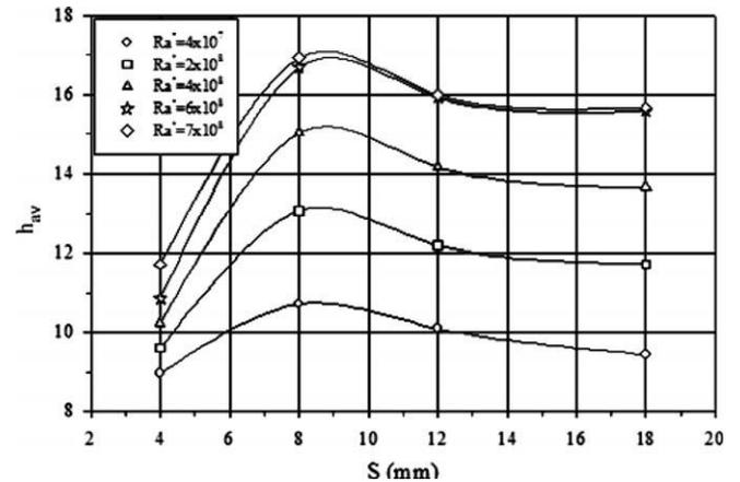
Fig. 14. Variation of average convection heat transfer coefficient with fin spacing (fin height,  $H_f/H = 0.50$ ).
