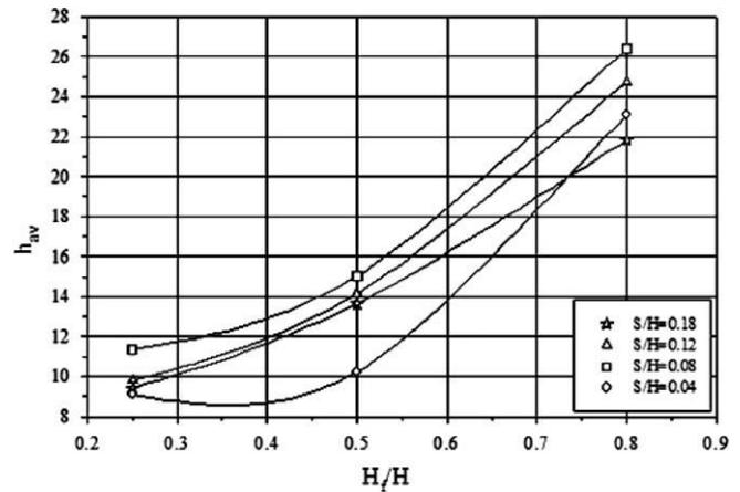
Fig. 10. Variation of average convection heat transfer coefficient with fin height at different fin spacings (average modified Rayleigh number,  $Ra^* = 4 \times 10^8$ ).
