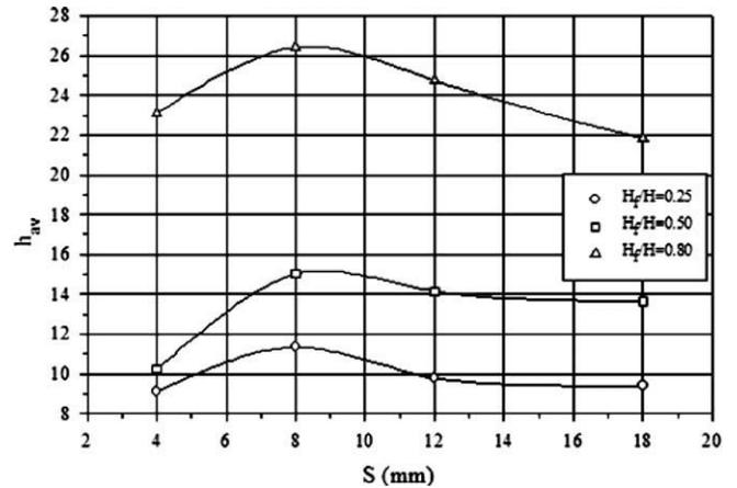
**Fig. 5.** Variation of average convection heat transfer coefficient with fin spacing at different fin heights (average modified Rayleigh number,  $Ra^* = 4 \times 10^8$ ).
