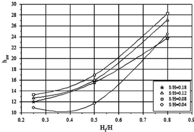
Fig. 12. Variation of average convection heat transfer coefficient with fin height at different fin spacings (average modified Rayleigh number,  $Ra^* = 7 \times 10^8$ ).
