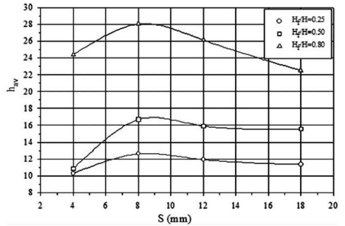
**Fig. 6.** Variation of average convection heat transfer coefficient with fin spacing at different fin heights (average modified Rayleigh number,  $Ra^* = 6 \times 10^8$ ).
