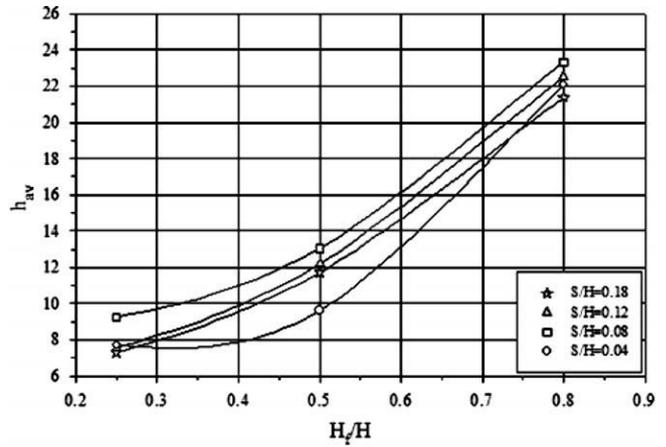
Fig. 9. Variation of average convection heat transfer coefficient with fin height at different fin spacings (average modified Rayleigh number,  $Ra^* = 2 \times 10^8$ ).
