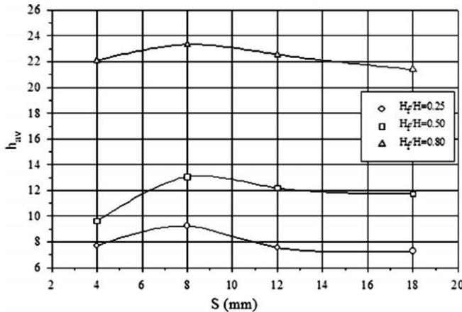
**Fig. 4.** Variation of average convection heat transfer coefficient with fin spacing at different fin heights (average modified Rayleigh number,  $Ra^* = 2 \times 10^8$ ).
