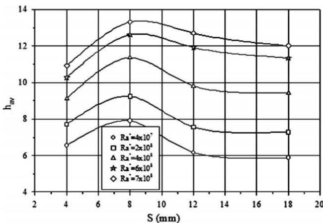
Fig. 13. Variation of average convection heat transfer coefficient with fin spacing (fin height,  $H_f/H = 0.25$ ).
