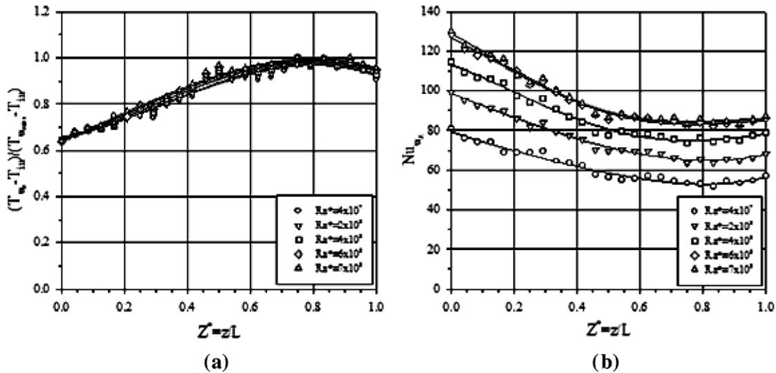
Fig. 17. (a) Variation of the temperature distribution and (b) variation of Nusselt Number with the main flow direction ( $z$ ) ( $S/H = 0.08$  and  $H_f/H = 0.50$ ).
