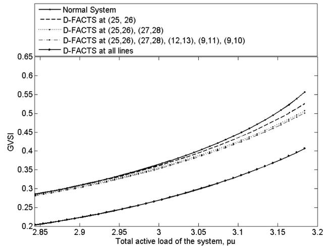
Fig. 3. Variation of GVSI for different operating conditions
