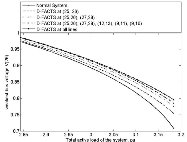
Fig. 4. Variation in weakest bus voltage for different operating conditions
