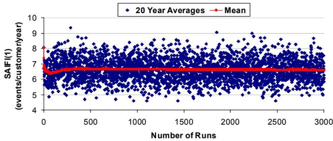
Figure 7. Determining SAIFI(1h) Convergence Value
