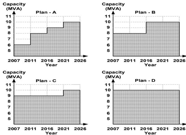
Figure 6. Different ESS Expansion Plans
