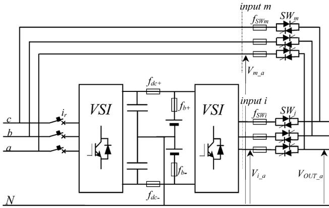
Fig. 3. Double conversion UPS with its protection devices. Voltages  $V_m$ ,  $V_i$ , and  $V_{out}$  pertaining to phase “a” of the system are also shown.
