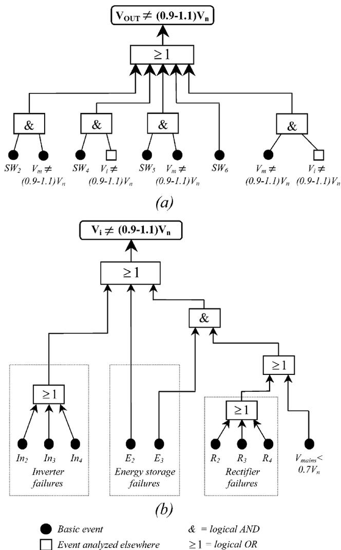
Fig. 4. (a) Static transfer switch fault tree. (b) UPS compensator fault tree.
