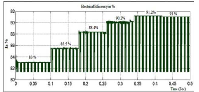
Fig. 21. Electrical Efficiency at different loads for Generic HPS architecture.
