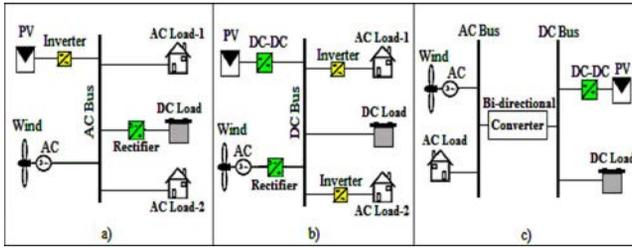
Fig. 1. Different architectures of standalone HPS.
