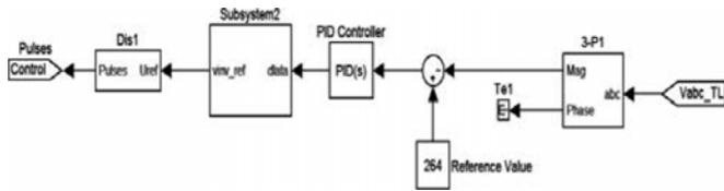
Fig. 9. MATLAB/Simulink model of Inverter firing pulses.
