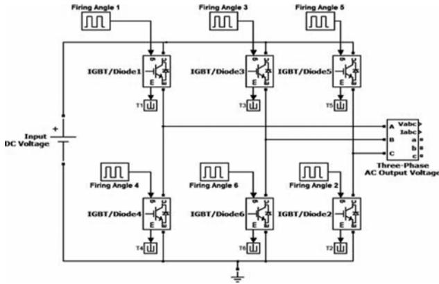
Fig. 8. MATLAB/Simulink model of Inverter.
