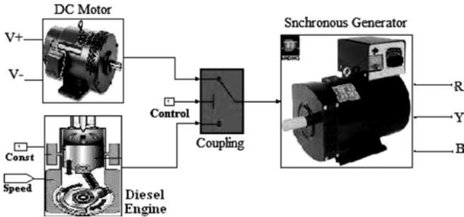
Fig. 10. MATLAB/Simulink model of dc motor/Diesel engine-Synchronous generator set.
