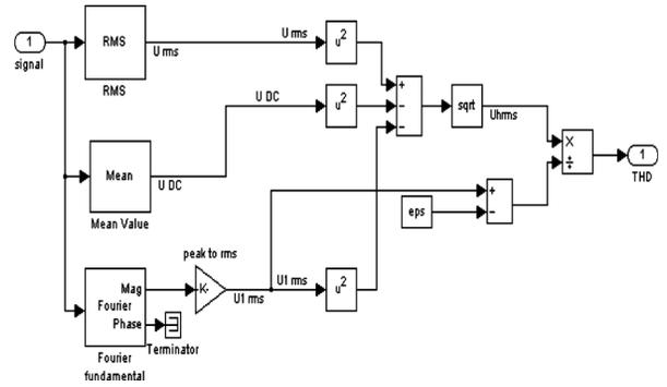
Fig. 16. Matlab/Simulink Modeling of THD block.
