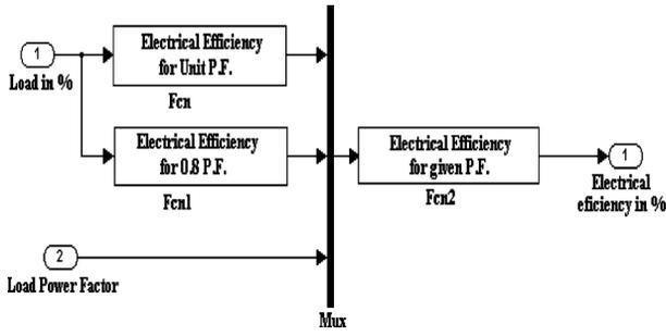
Fig. 19. Matlab/Simulink Model for electrical efficiency.
