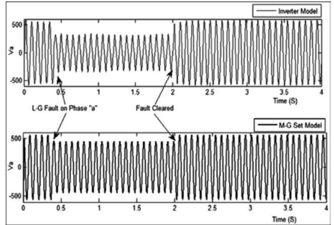
Fig. 24. Comparison of Voltage Sag of faulted phase for both generic and retrofitted HPS systems.
