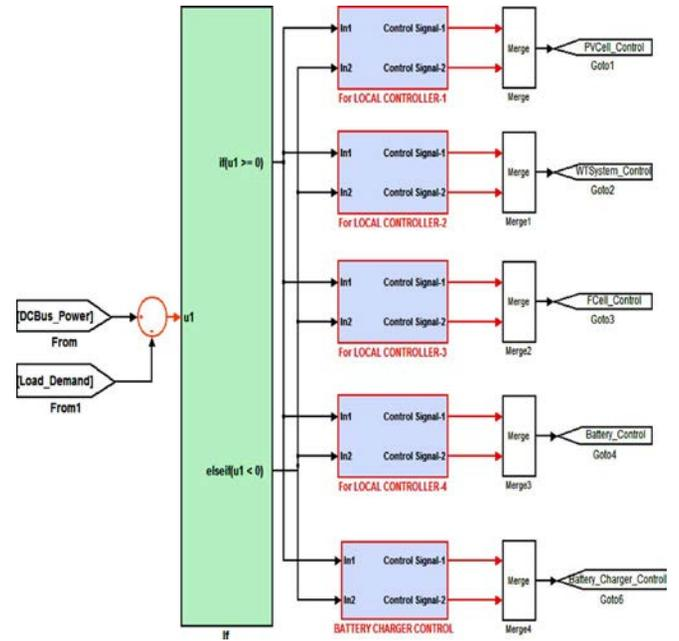
Fig. 15. MATLAB/Simulink model of EMCU.
