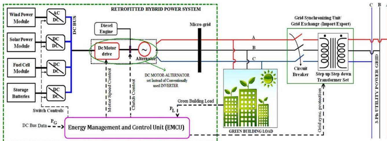
Fig. 4. The architecture of the retrofitted HPS connected to the building and running in parallel with utility grid.
