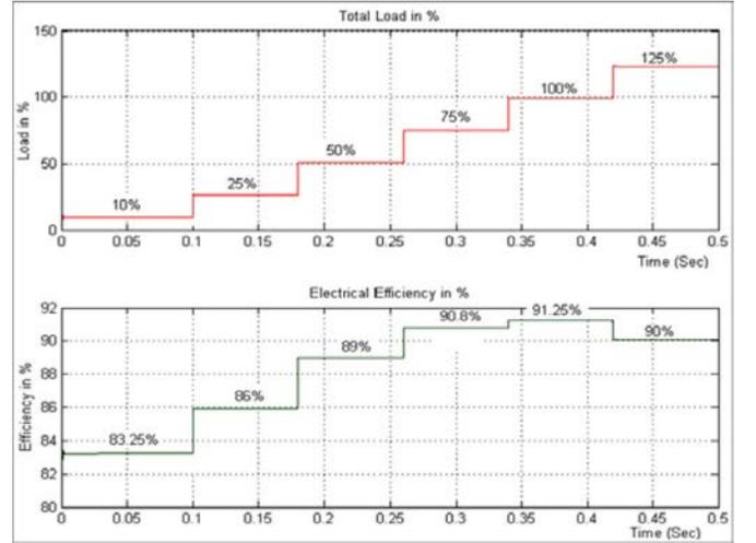
Fig. 20. Electrical Efficiency at different loads for retrofitted HPS architecture.
