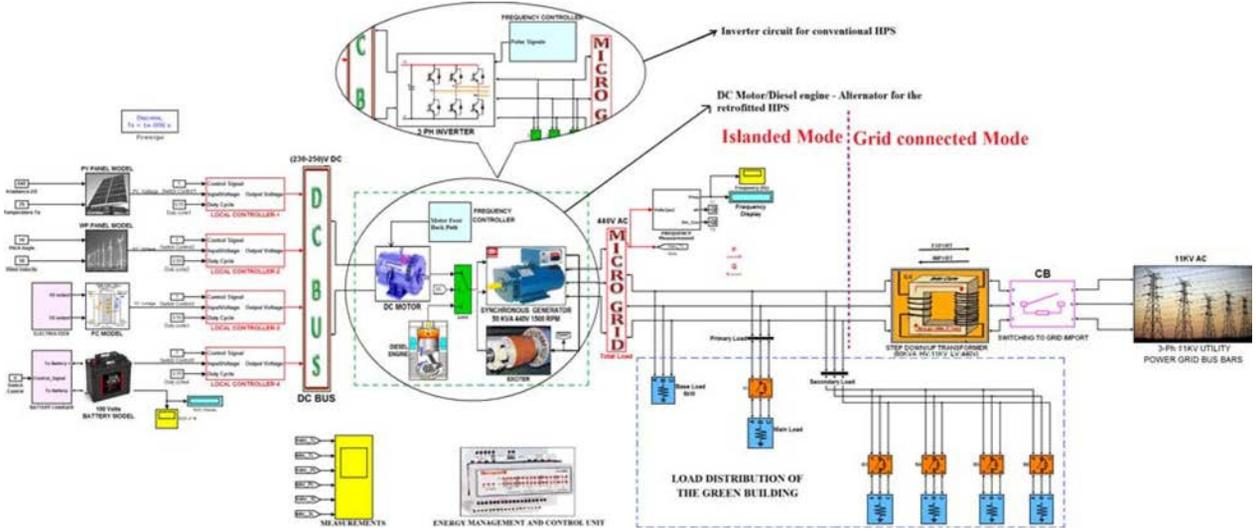
Fig. 13. MATLAB/Simulink model of the proposed retrofitted Hybrid Power System architecture for buildings.
