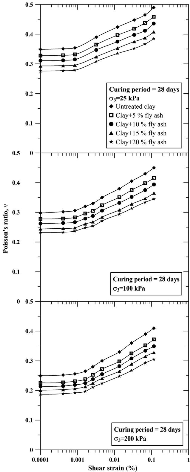
**Fig. 7.** Variation of Poisson's ratio ( $\nu$ ) with shear strain for a 28-day curing period
