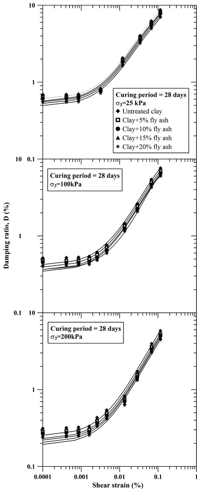
**Fig. 5.** Variation of damping ratio ( $D$ ) with shear strain for a 28-day curing period
