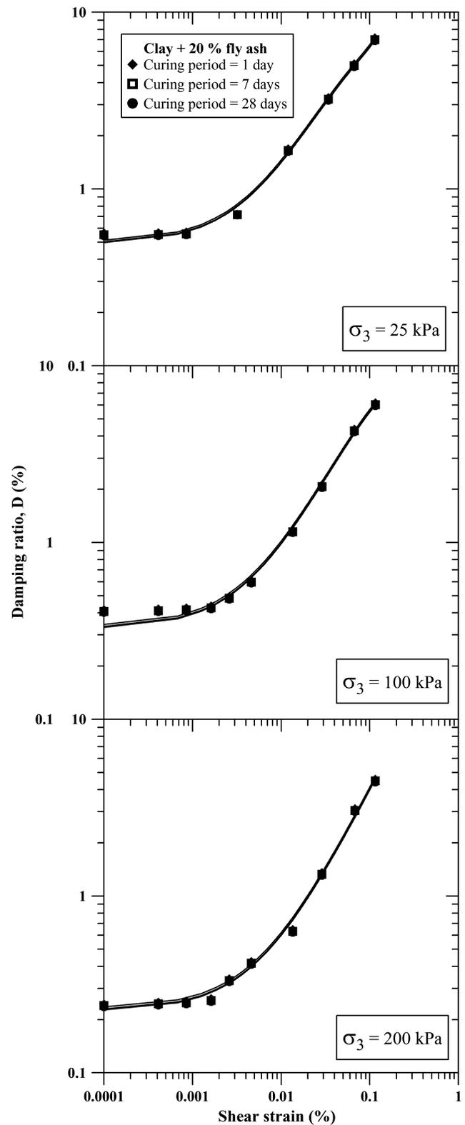
**Fig. 6.** Variation of damping ratio ( $D$ ) with shear strain for different curing periods
