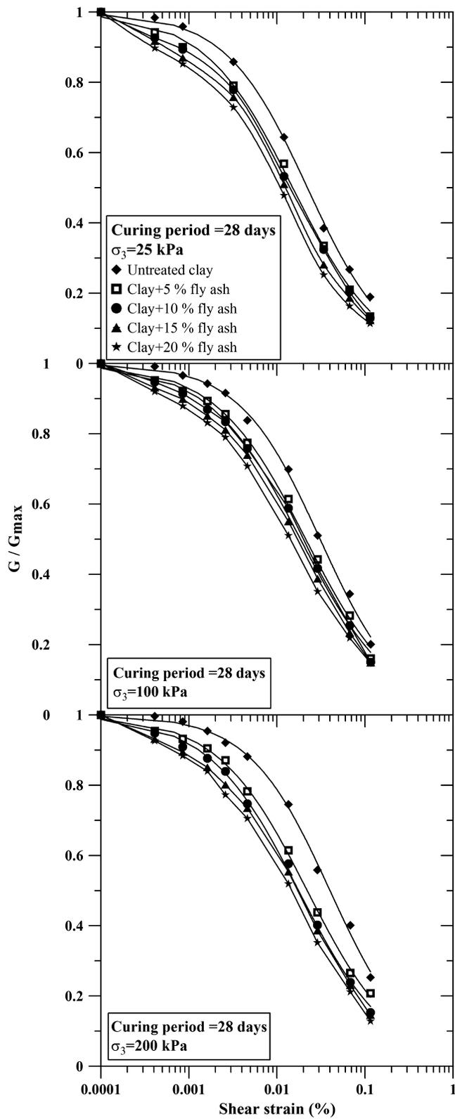
**Fig. 2.** Variation of modulus degradation ( $G/G_{max}$ ) with shear strain for a 28-day curing period
