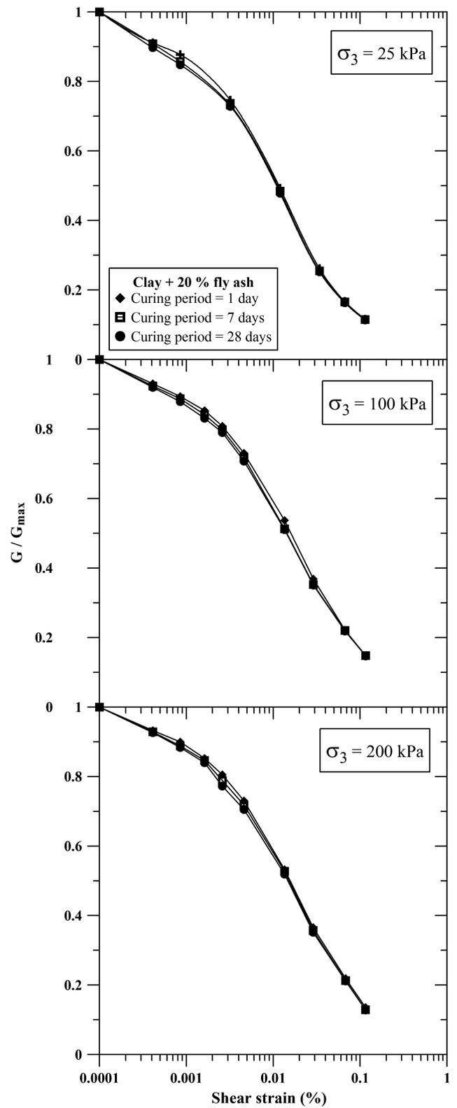
**Fig. 3.** Variation of modulus degradation ( $G/G_{max}$ ) with shear strain for different curing periods
