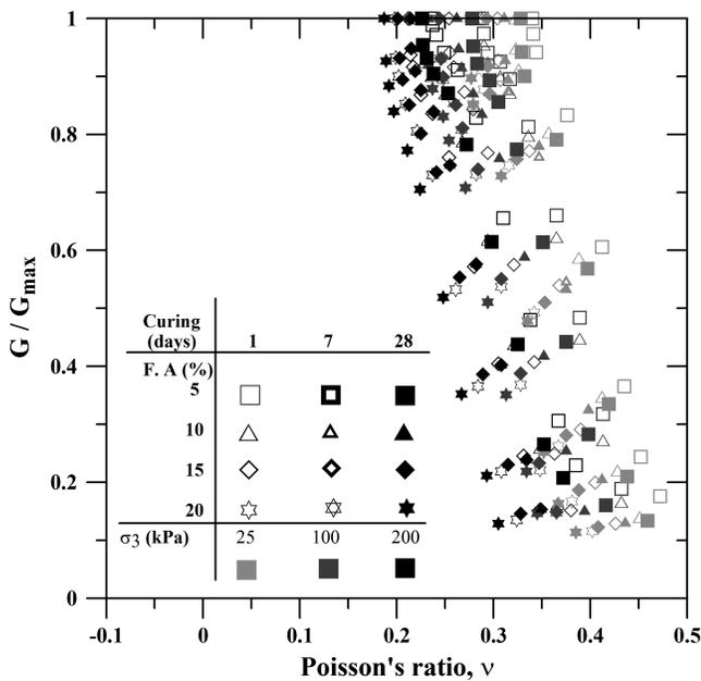
**Fig. 9.** Variation of Poisson's ratio with normalized shear modulus
