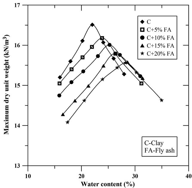
Fig. 1. Compaction characteristics of treated and untreated clay
