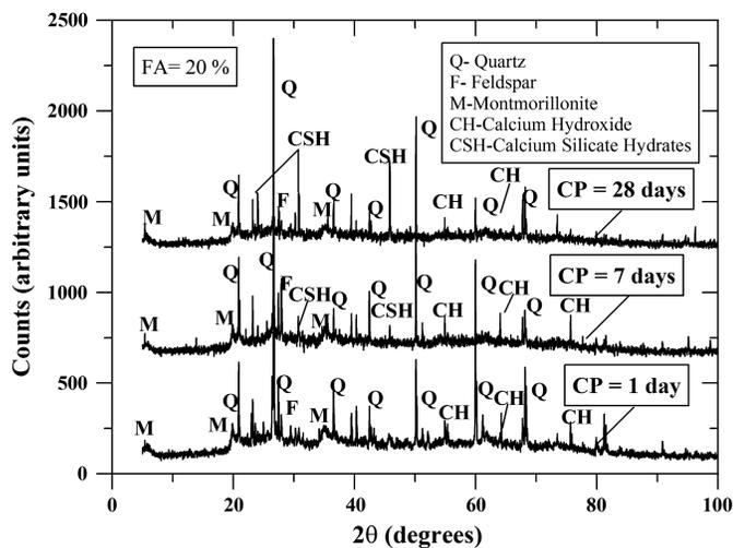
Fig. 12. XRD results of samples treated with 20% fly ash for different curing periods
