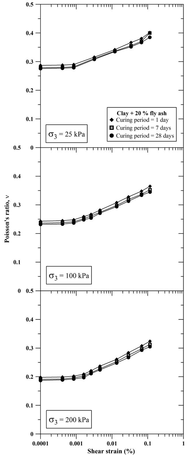
**Fig. 8.** Variation of Poisson's ratio ( $\nu$ ) with shear strain for different curing periods
