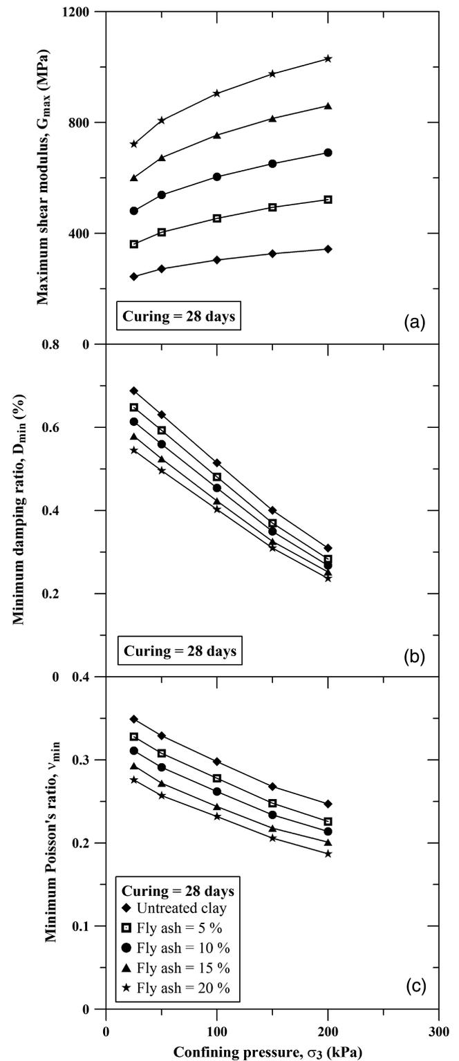
**Fig. 10.** Variation of small-strain dynamic properties with confining pressure: (a) shear modulus ( $G_{\max}$ ); (b) damping ratio ( $D_{\min}$ ); (c) Poisson's ratio ( $\nu_{\min}$ )
