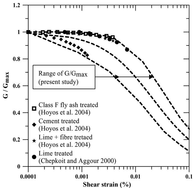
**Fig. 4.** Validation of normalized modulus degradation ( $G/G_{max}$ ) upper and lower bound curves
