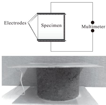
Fig.2 The two-electrode method
