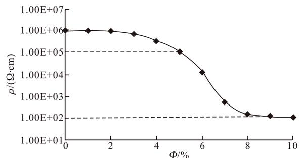
Fig.3 Calculated resistivity with different carbon black contents
