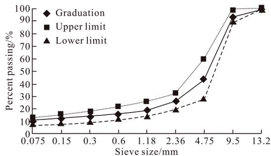
Fig.1 Gradation of aggregate
