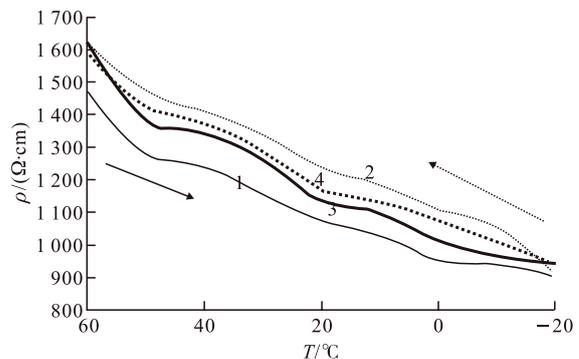
Fig.8 Resistivity-temperature characteristics in temperature cycle ( $\phi=6.7\%$ )
