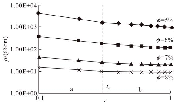
Fig.5 Resistivity with different relative temperature  $t$
