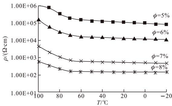
Fig.4 Resistivity-temperature characteristics with different carbon black contents
