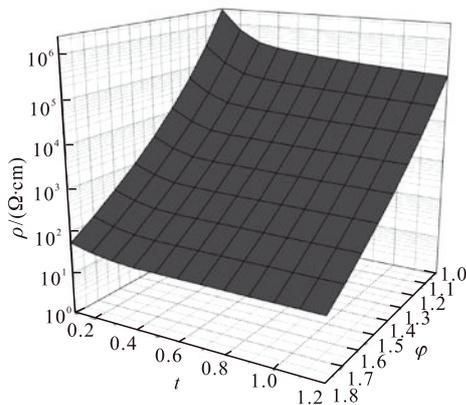
Fig.7 Resistivity with the changes of temperature and the carbon black content
