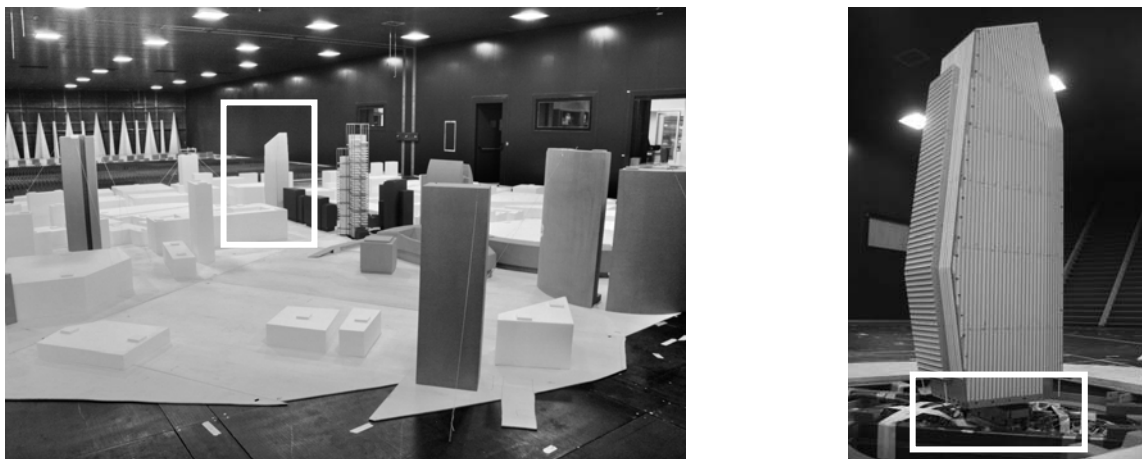
Figure 1. Test arrangement. The model of the tower and the surrounding in the wind tunnel test section (sx). Close up view of the tower and the force balance (dx).
