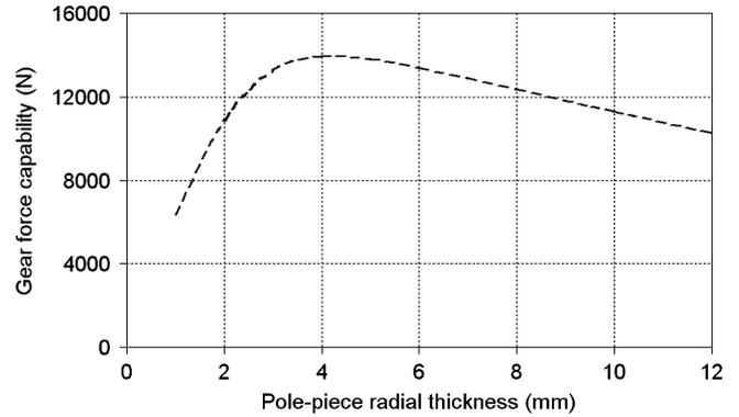
Fig. 6. Variation in force capability with pole-piece radial thickness.
