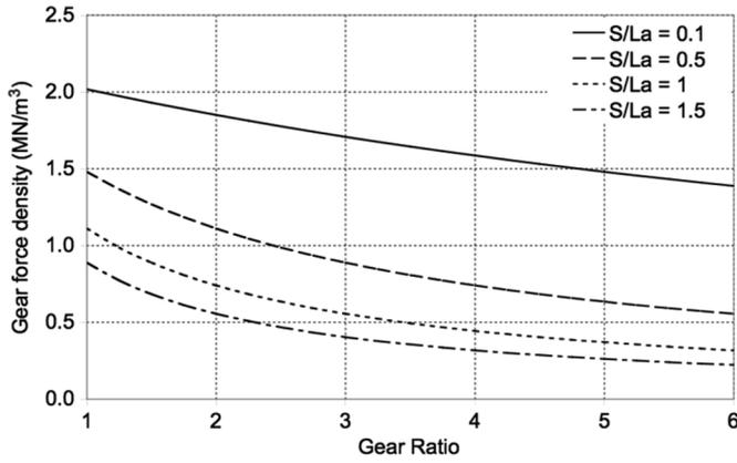
Fig. 2. Variation of gear force density with gear ratio.
