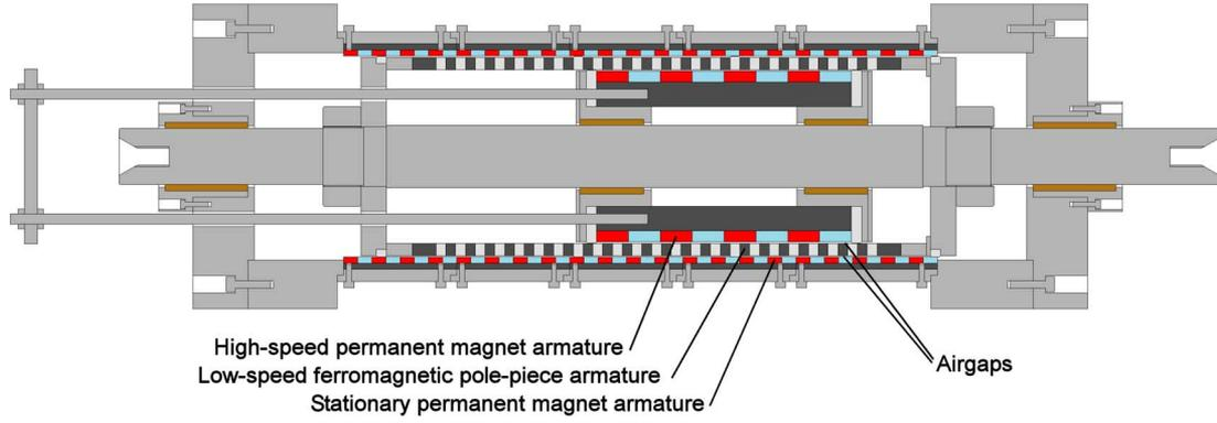
Fig. 1. Cross-sectional schematic of the prototype linear magnetic gear.
