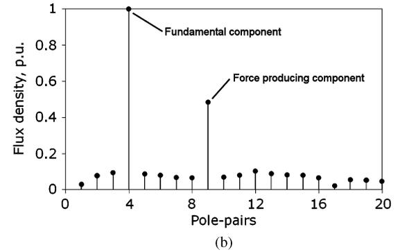
Fig. 4. Radial flux density in the airgap adjacent to the stationary armature due to high-speed armature magnets. (a) Flux density waveform. (b) Harmonic spectrum with pole pieces.
