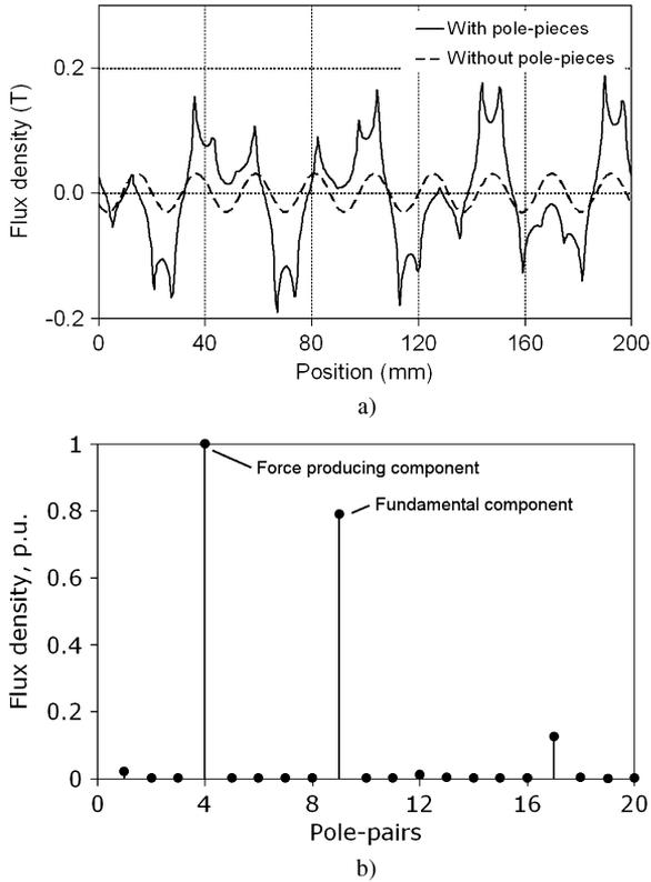
Fig. 5. Radial flux density in the airgap adjacent to the high-speed armature due to stationary armature magnets. (a) Flux density waveform. (b) Harmonic spectrum with pole pieces.
