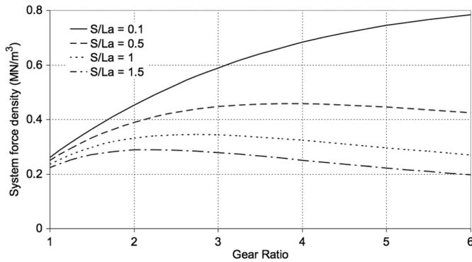
Fig. 3. Variation of system force density with the gear ratio.
