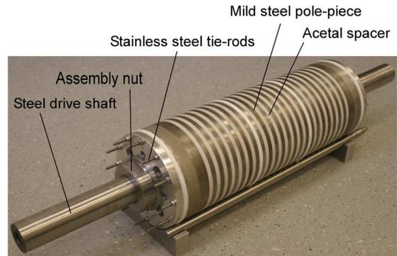
Fig. 8. Pole-piece armature with an integrated high-speed armature.
