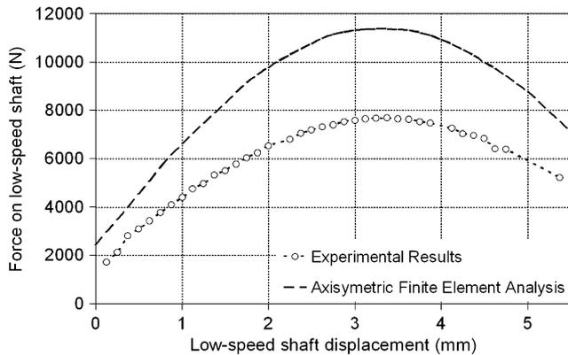
Fig. 10. Variation of measured and predicted force on the pole-piece armature with position. (Locked high-speed armature).
