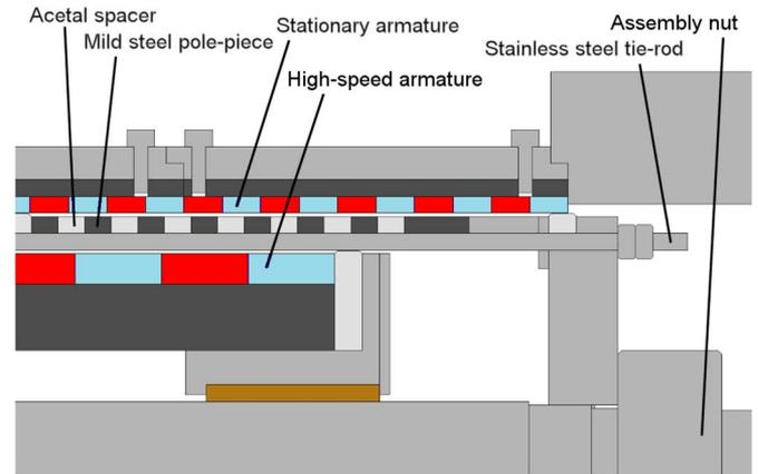
Fig. 7. Schematic of magnetic gear (a close-up view).
