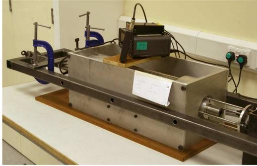
Fig. 9. Magnetic gear on the test bed.
