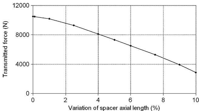
Fig. 11. Variation of transmitted force with the change of axial distance between the pole-piece rings.
