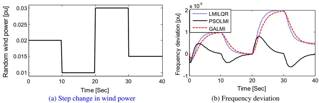
Fig. 7. Response for case study-1 with step change in wind power.
