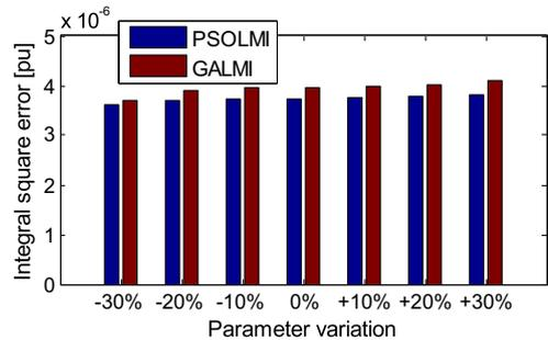
Fig. 16. Computed ISE for change in all system parameters.
