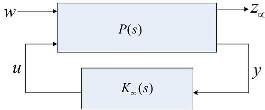
Fig. 1. Closed-loop system via robust  $H_\infty$  control.
