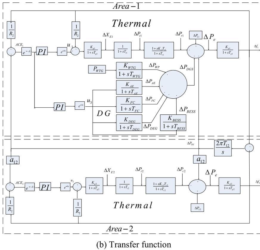
Fig. 3. Case study-2: two area power system with DG.
