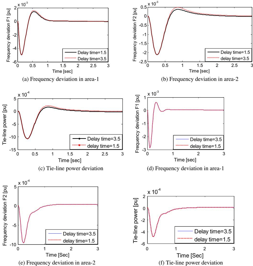
Fig. 15. Response for case study-2 with time delays.
