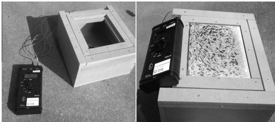
Fig. 3. Translucency measurement test set-up.
