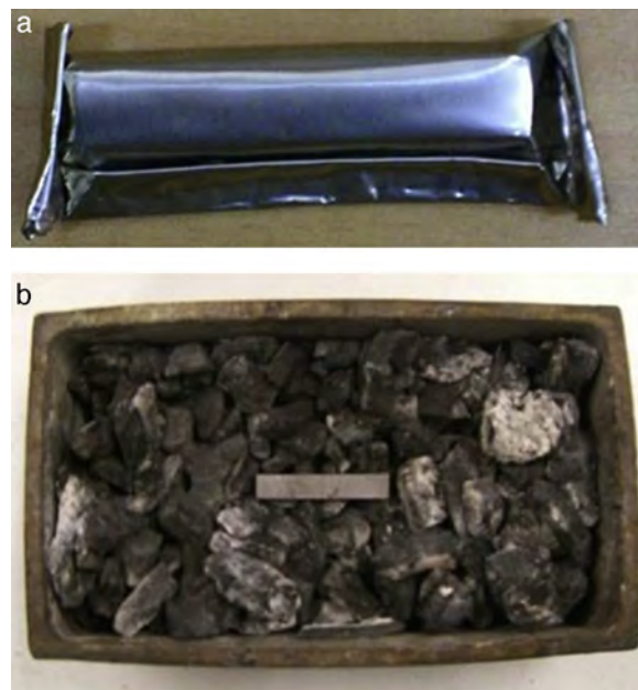
Fig. 1 – (a) Stainless steel foil wrapping and (b) pack carburization.
