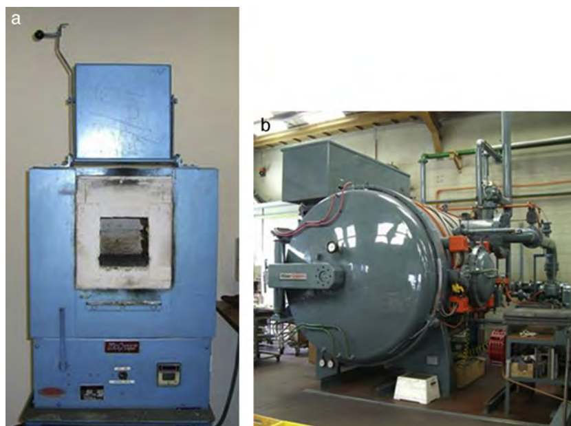
Fig. 2 – Furnaces used for heat treatment hardening experiments: (a) muffle furnace and (b) vacuum furnace.
