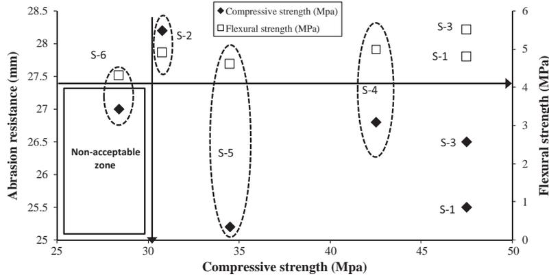
**Fig. 3.** Relationship of flexural/compressive strength with abrasion resistance value at 28 days.
