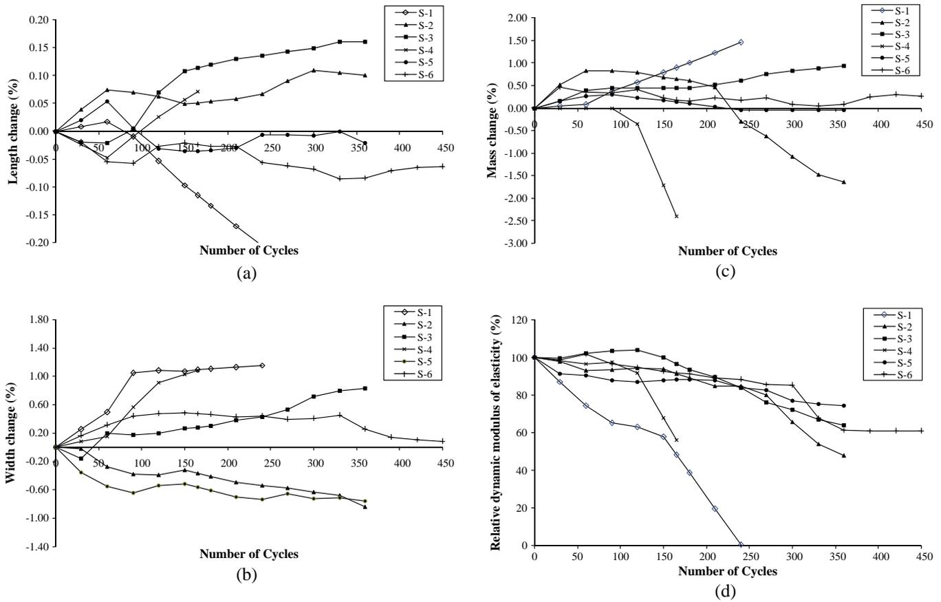
Fig. 4. (a) Length change, (b) width change, (c) mass change and (d) relative dynamic modulus of elasticity vs. the number of cycles for mixtures.
