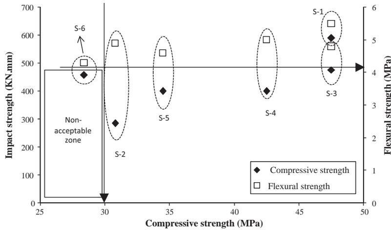
**Fig. 2.** Relationship of flexural/compressive strength with impact strength at 28 days.
