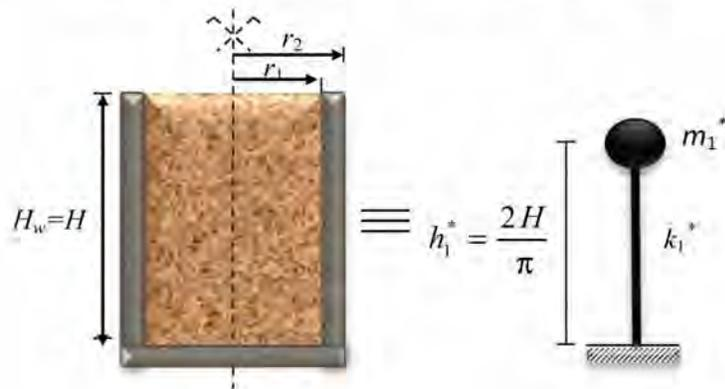
$$k_s = \frac{3E_w \pi (r_2^4 - r_1^4)}{4H_w^3} + \frac{3E_m \pi r_1^4}{4H^3} \quad (6)$$
