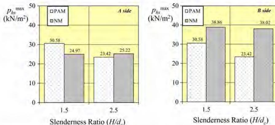
**Fig. 10** Maximum dynamic material pressure variations for two different slenderness ratios according to PAM and NM
