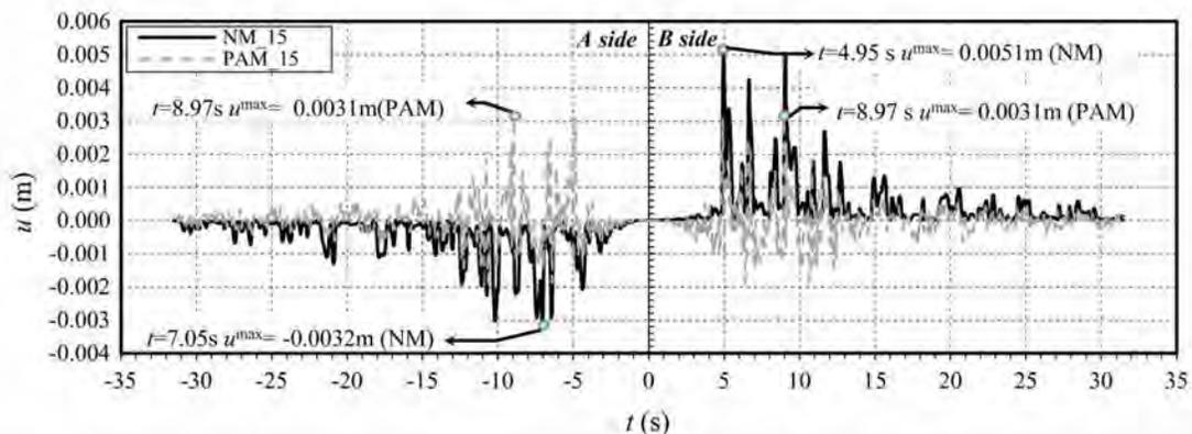
**Fig. 11** Variations of horizontal displacements in time at opposite sides of the wall in the earthquake direction for PAM\_15 and NM\_15
