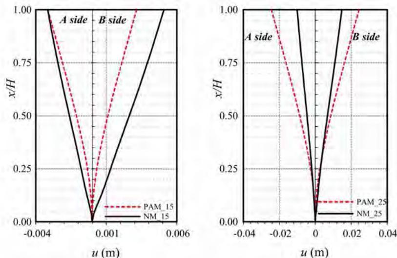
**Fig. 13** Comparisons of the maximum horizontal displacements throughout the height of the silo for two different slenderness ratios via PAM and NM
