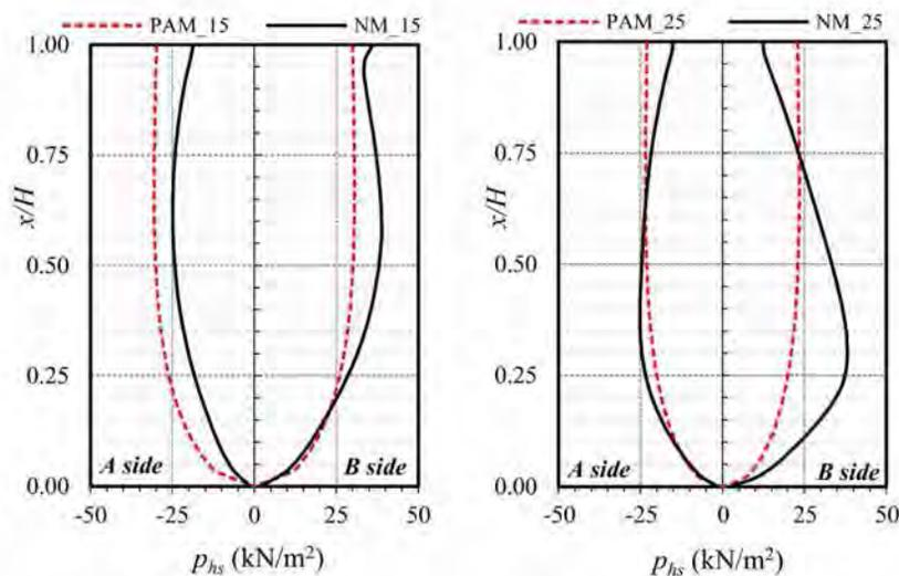
**Fig. 9** Comparisons of the maximum dynamic pressures throughout the height of the silo for two different slenderness ratios via PAM and NM
