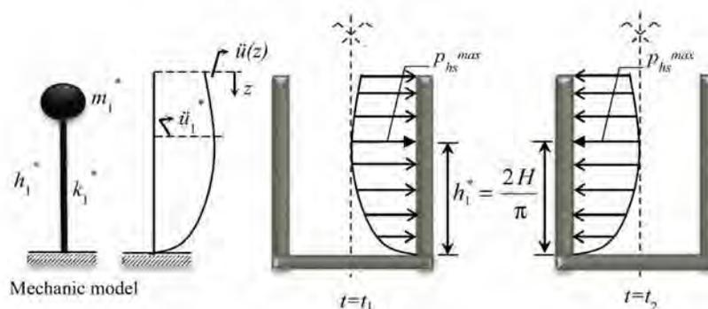
**Fig. 5** The distribution of dynamic material pressures along the height of the silo
