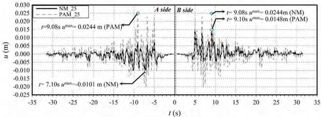
**Fig. 12** Variations of horizontal displacements in time at opposite sides of the wall in the earthquake direction for PAM\_25 and NM\_25
