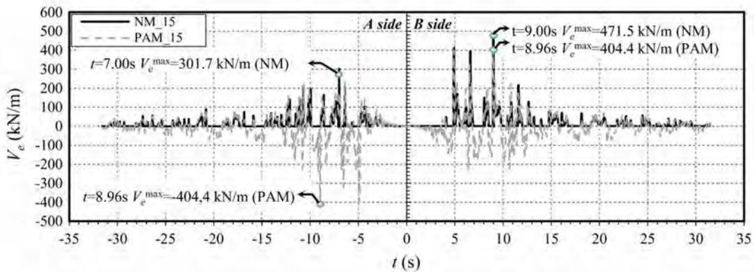
**Fig. 15** Variations of equivalent base shears in time at opposite sides of the silo wall in the earthquake direction for slenderness ratio 1.5 via PAM and NM
