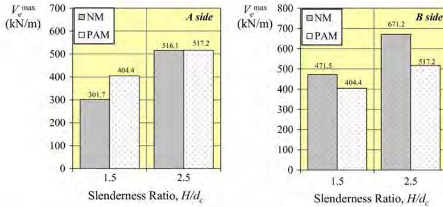
**Fig. 14** Maximum equivalent base shears for two different slenderness ratios at the opposite sides of the silo wall in earthquake direction via PAM and NM
