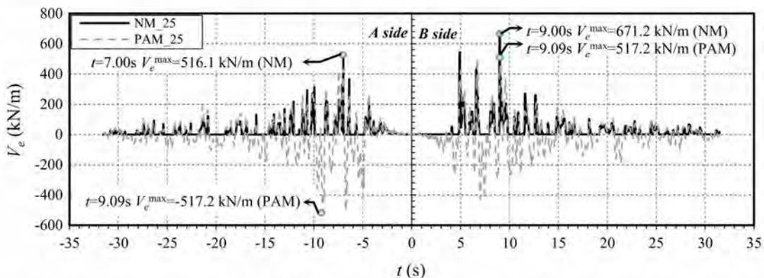
**Fig. 16** Variations of equivalent base shears in time at opposite sides of the silo wall in the earthquake direction for slenderness ratio 2.5 via PAM and NM
