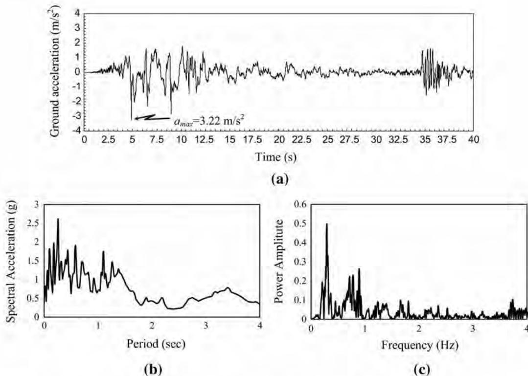
**Fig. 8** Acceleration time history (a), response spectrum (b) and power spectrum (c) of N–S component of Yarimca Station–Izmit Earthquake
