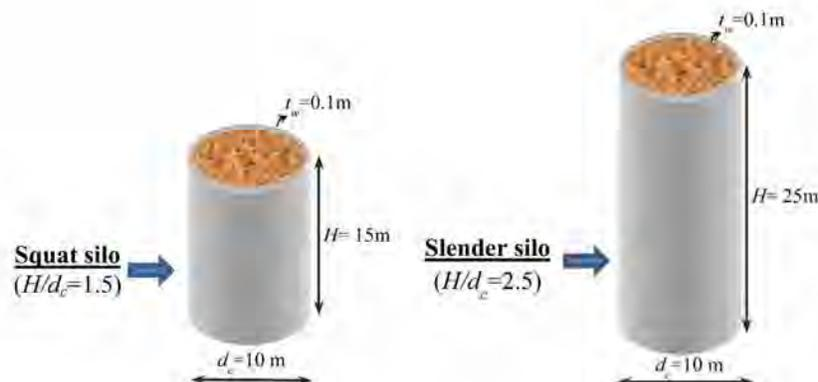
**Fig. 7** Geometrical properties of considered silos
