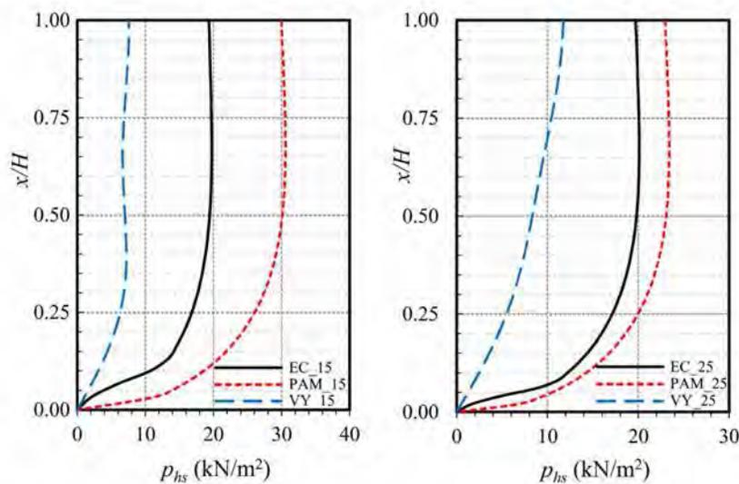
**Fig. 18** Comparison of the maximum dynamic material pressure along the height of the silo wall for two different slenderness ratios via VY, EC and PAM
