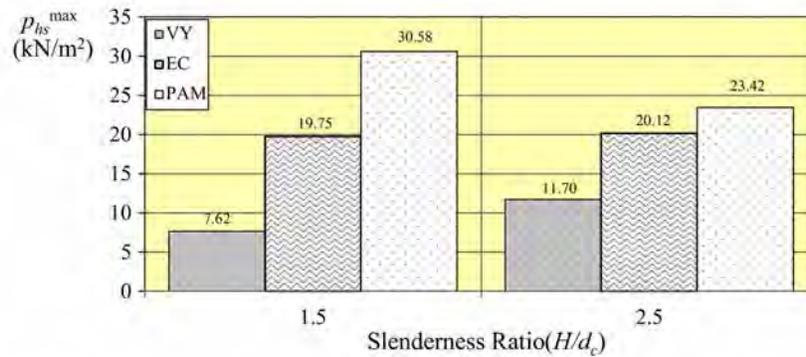
**Fig. 17** Maximum dynamic material pressures for two different slenderness ratios via PAM, EC and VY
