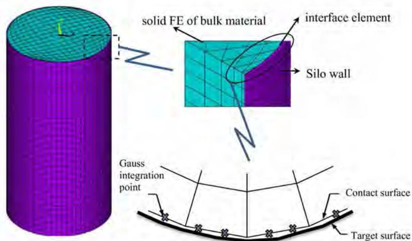
**Fig. 6** Finite element models for silos (Durmuş 2013)
