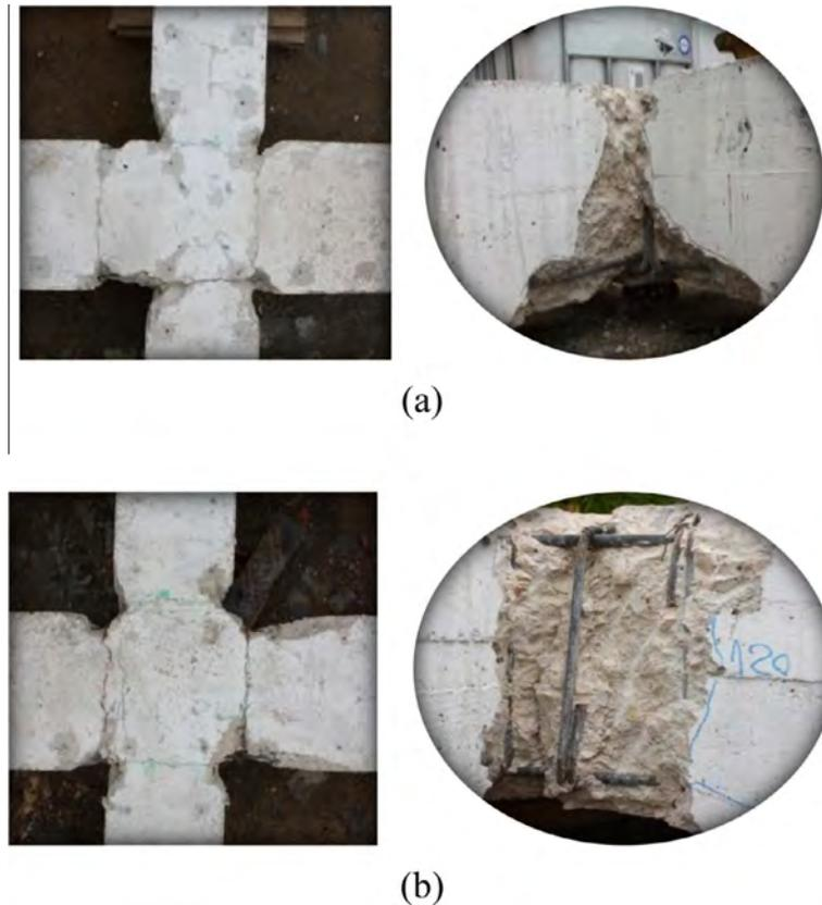
Fig. 4. The extent of damages before retrofitting (a) JPA0 and (b) JPC.
