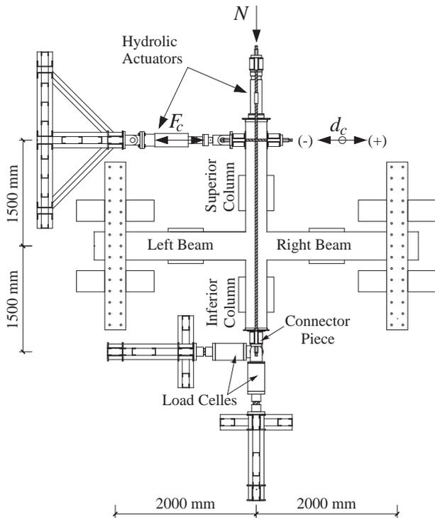
Fig. 3. Test setup for the horizontally placed specimens [21].
