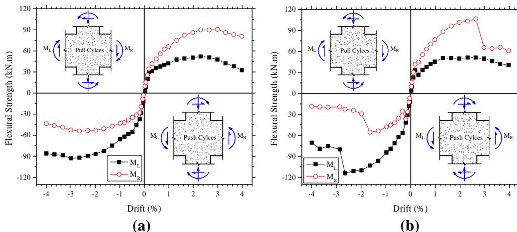
Fig. 11. Development of the resisting bending moment at the interfaces of the beams with columns (the positive moment is assumed as the anticlockwise rotation) for specimen (a) JPA0-R and (b) JPC-R.
