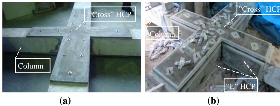
Fig. 6. View of the repaired specimens (a) JPA0-R and (b) JPC-R.
