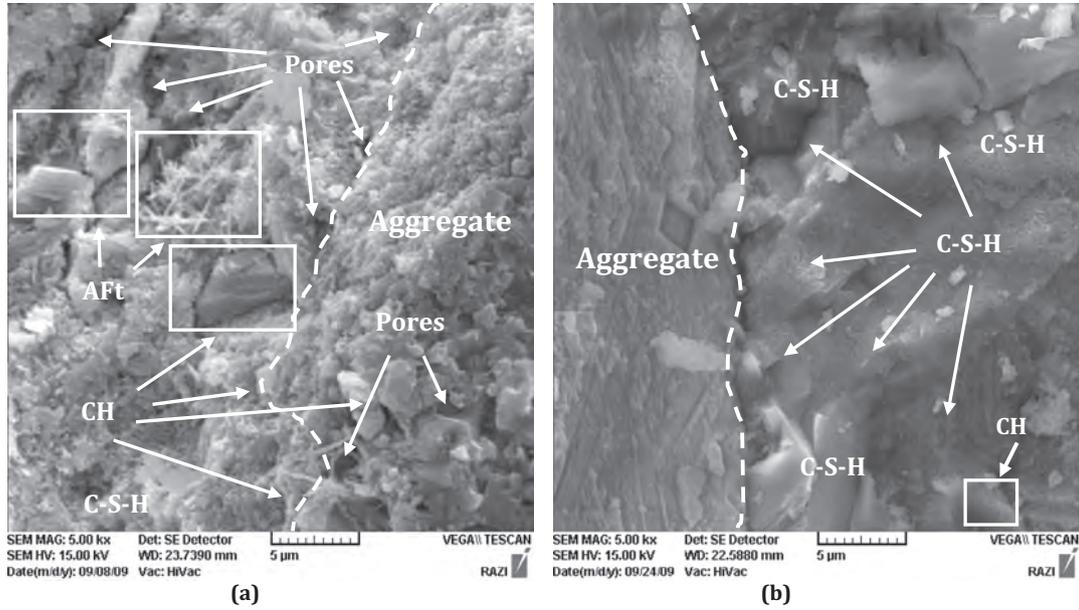
Fig. 6. The SEM micrographs of the ITZ between the aggregate and bulk cement paste for (a) the reference concrete (NS0-Ref) and (b) the sample incorporating 3% nS (NS3-Ref).
