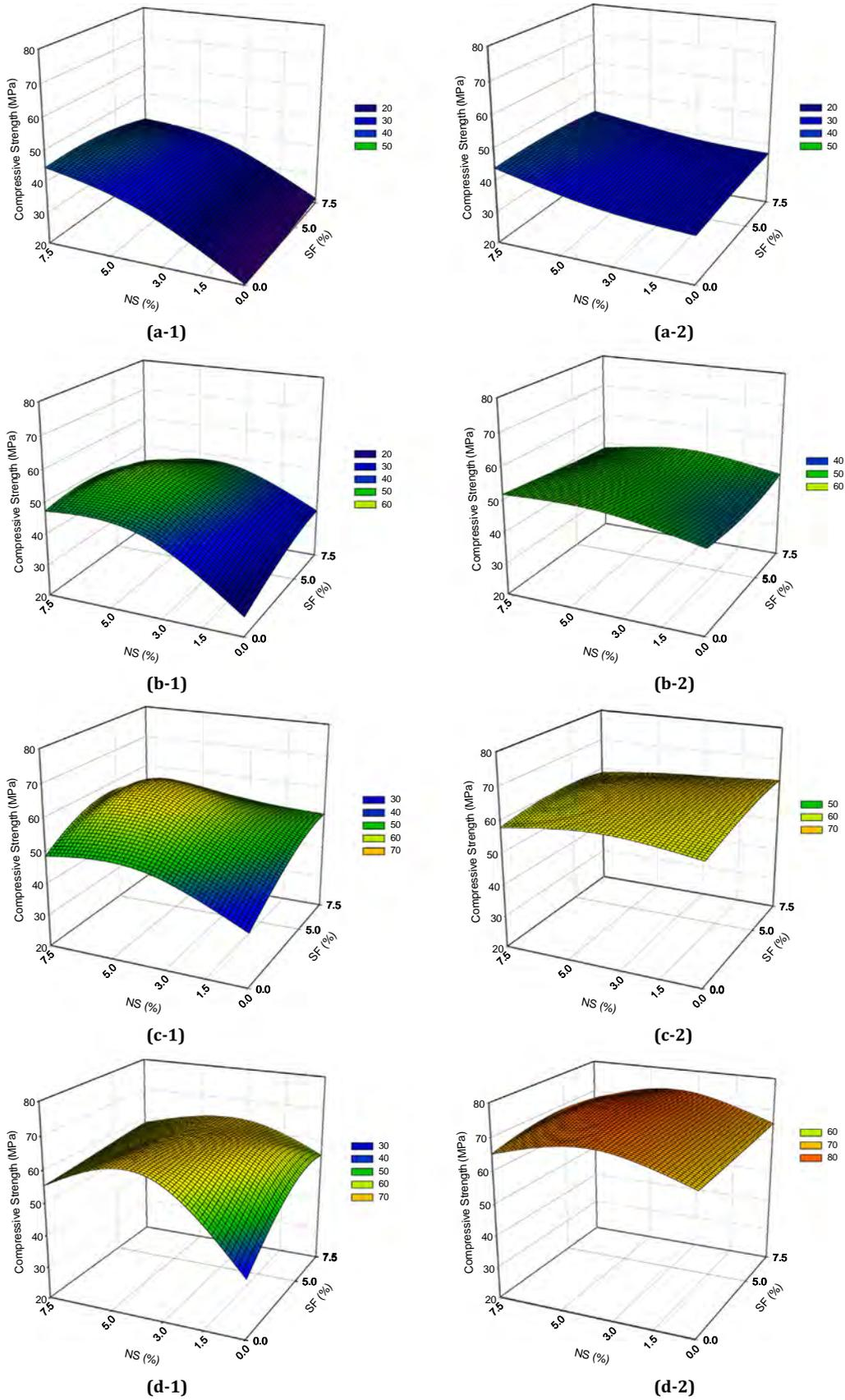
Fig. 3. Compressive strength of (1) cement paste and (2) concrete specimens as a function of nS and SF contents at (a) 3, (b) 7, (c) 28 and (d) 91 days.
