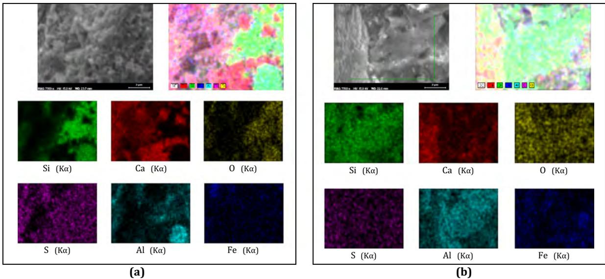
Fig. 8. The images of the elemental analysis by EDS color-mapping-scan corresponding to the SEM images of the ITZ for (a) the reference concrete (NS0-Ref) and (b) the sample incorporating 3% nS (NS3-Ref). (For interpretation of the references to colour in this figure legend, the reader is referred to the web version of this article.)
