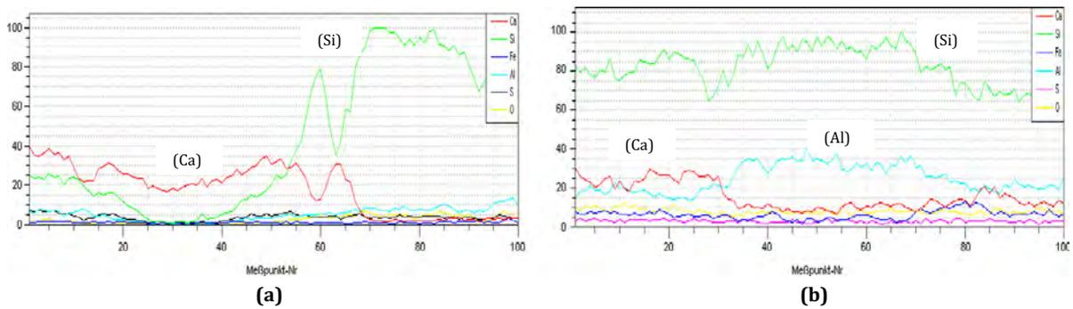
Fig. 7. The profiles of elemental analysis by EDS line-scan corresponding to the SEM images of the ITZ for (a) the reference concrete (NS0-Ref) and (b) the sample incorporating 3% nS (NS3-Ref).
