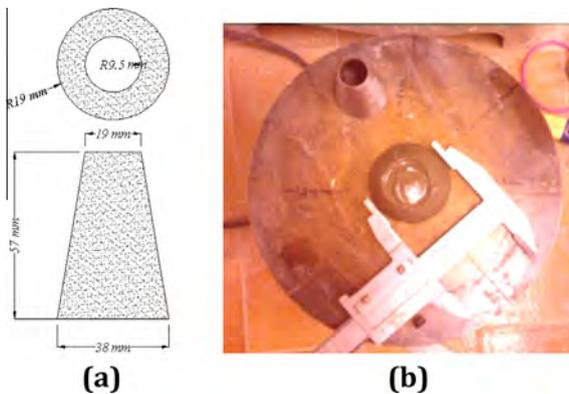
**Fig. 2.** Mini-slump cone (a) schematic shape and dimensions (b) measurement of spread.
