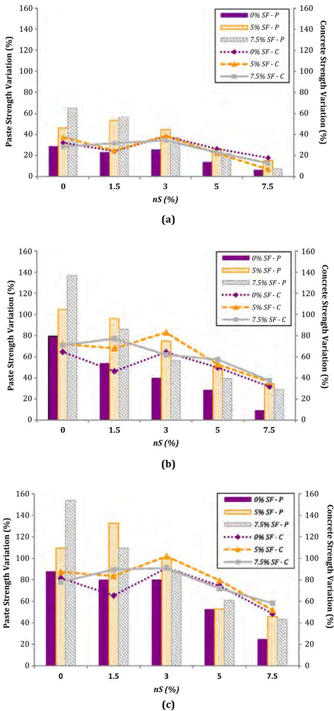
**Fig. 4.** Cement paste and concrete compressive strength variation percentage at (a) early age (3–7 days), (b) middle curing age (3–28 days) and (c) long-term (3–91 days) for mixtures incorporating 0%, 5% and 7.5% SF.
