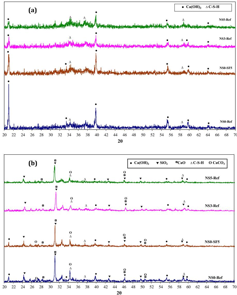
**Fig. 5.** XRD pattern of hardened (a) cement paste and (b) concrete, incorporating 0%, 3% and 5% nS (NS0-Ref, NS3-Ref and NS5-Ref) and 5% SF (NS0-SF5) at 28 days.
