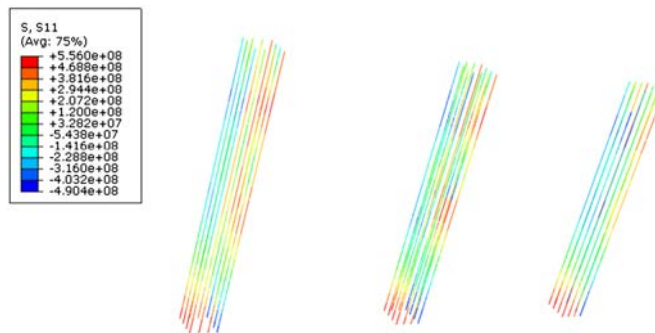
Figure 15. Distribution of stress of reinforcement of CESHRC (Step 8).
