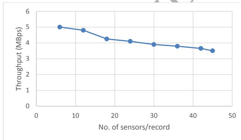
Figure 19, Throughput of the system by increasing the number of sensors per record for 1GB of data
