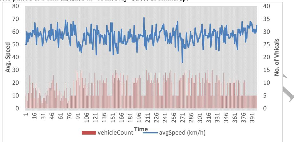
Figure 4. The speed of vehicles at low intensity of traffic between two points.
