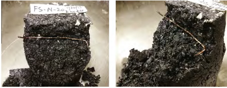
Fig. 5. Copper wire electrode in a sample after testing.
