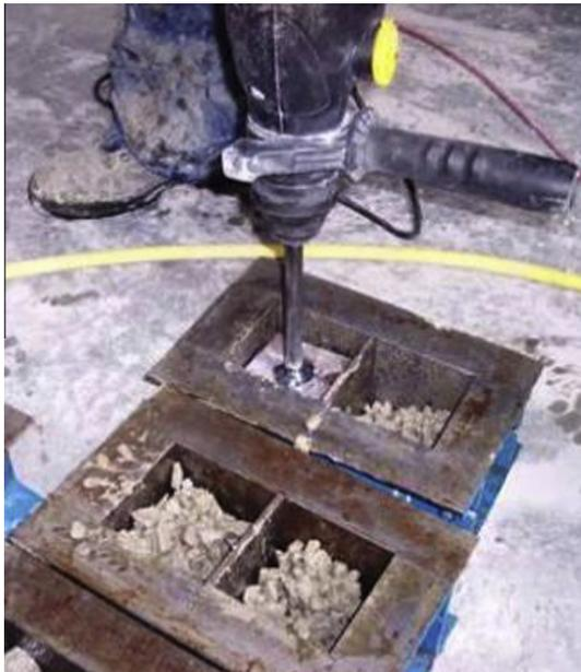
**Fig. 2.** Cast and compaction of no-fines concrete specimens.
