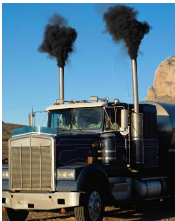
Emission of soot in the fumes of a large diesel truck, without particle filters
